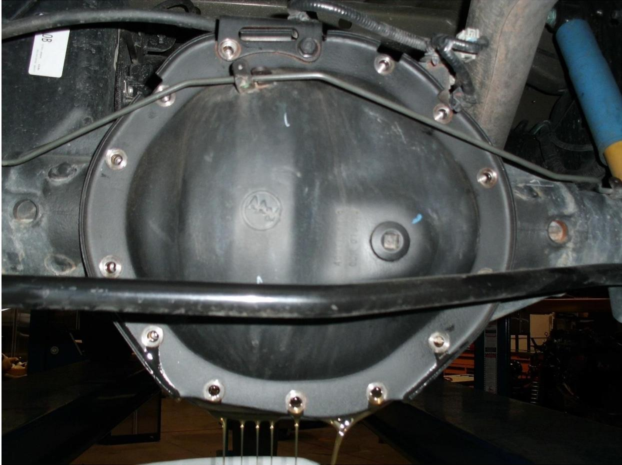
5. Remove the remaining bolt from the top of the differential cover.
