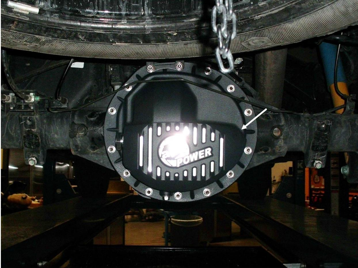
16. Using the top fill port, fill the aFe differential cover with new gear oil. Fill until gear oil runs out of the 1/8" NPT port on the side of the cover (about 3 ½ quarts).
