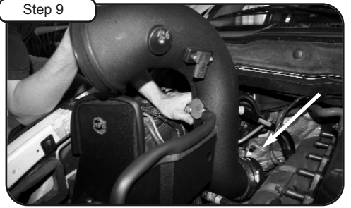
Step 9 Install hi-temp coupler with clamps provided to tube. Now install tube into vehicle.
