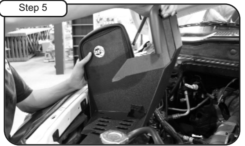
Step 5 Install 3/4" Trim seal to housing. Now install housing into vehicle.
