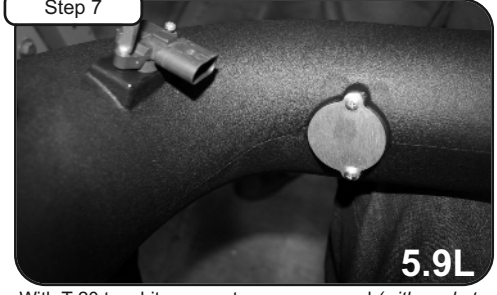
Step 7 With T-20 torx bit remove temp sensor and (with gasket and screws provided) install into new tube. (5.9L place MAF cover with gasket and tighten using short screws provided. Install plug into the hole in tube for crank case line.)
