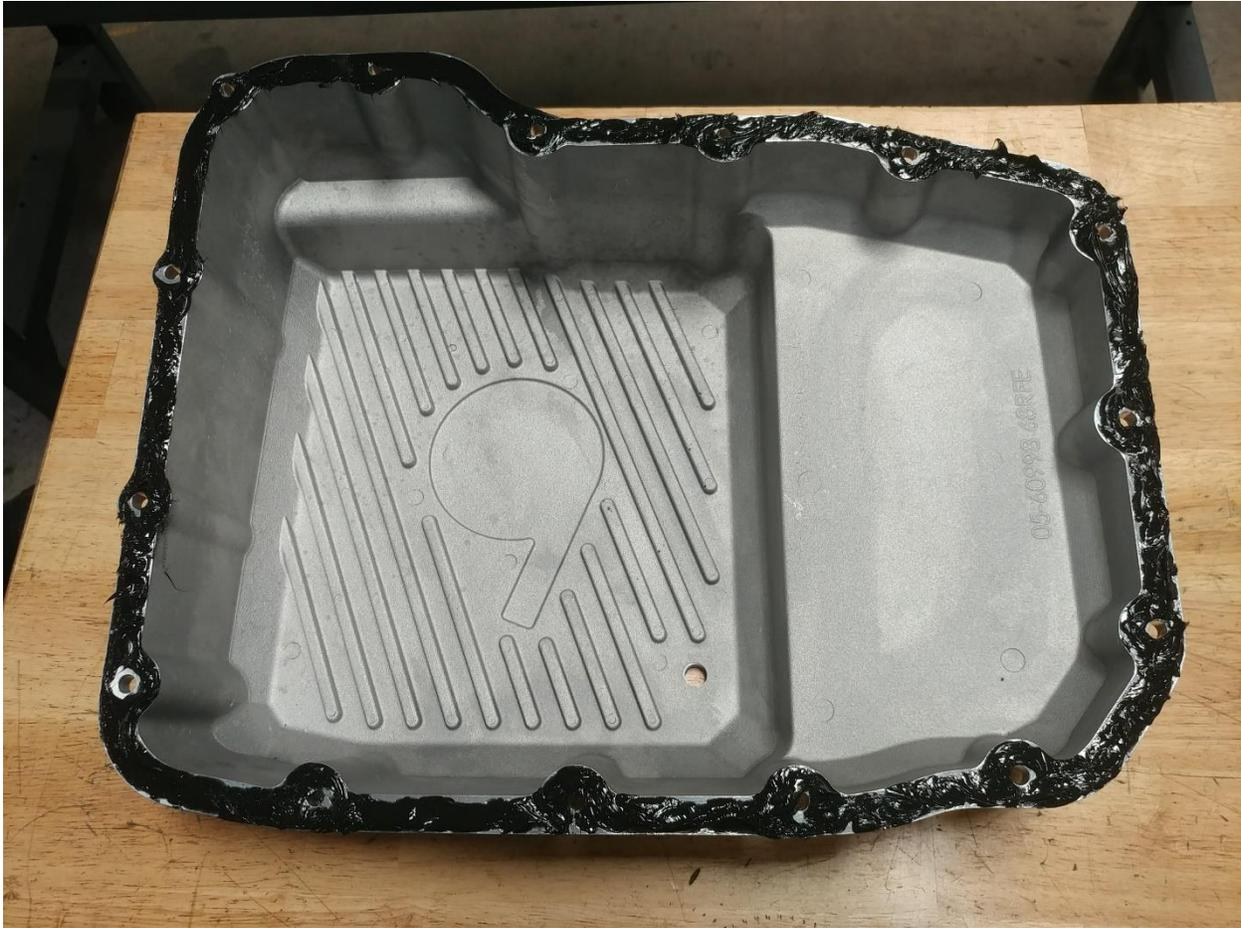
12. Hold the supplied aFe transmission pan up to the gasket surface to make sure you will be able to maneuver it into place. We recommend lifting the passenger side of the pan into place first.
