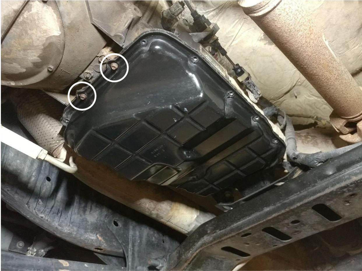
3. Remove 13 bolts from the transmission pan, leaving the front two (2) in place.
