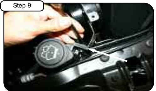
Using a 10mm wrench loosen bolt holding washer fluid reservoir. Place 5 1/2" adapter in to new housing and tighten using button head screws provided with 5/32 allen key. Install housing in to vehicle and re-tighten bolt.
