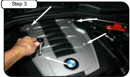
Remove the 4 bolts holding the factory engine cover with 10mm socket w/ ratchet. Remove engine cover.
