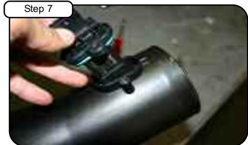
With provided T20 torx bit loosen the 2 bolts that hold in the MAF sensor. Carefully remove MAF sensor out.
