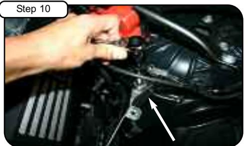
With OE T25 bolt, use to tighten new housing in to place. Tighten at bottom of housing using nut and washer provided with 10mm socket w/ extension.
