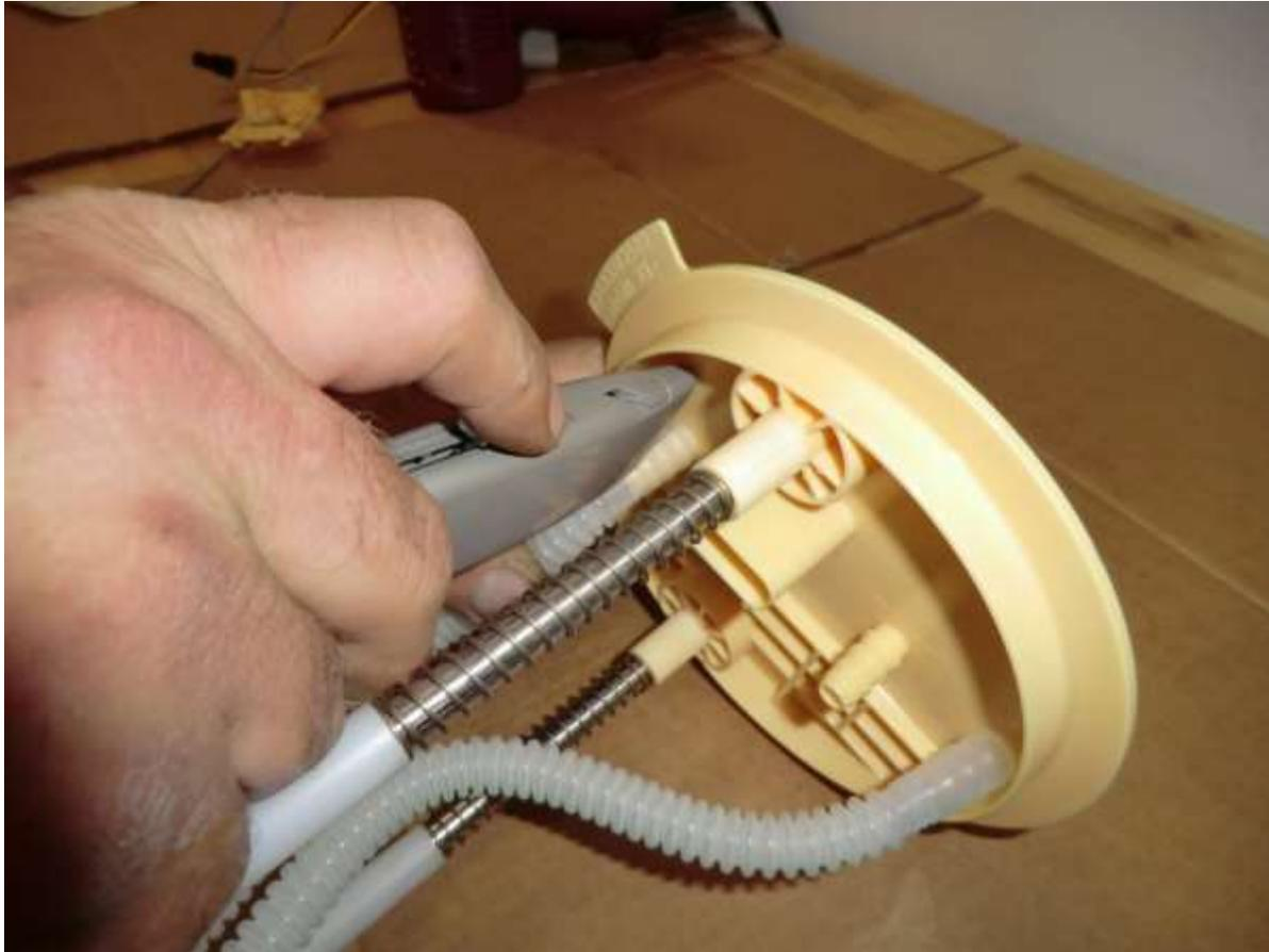
7. Unplug the electrical connector at the top of the fuel sender assembly.
