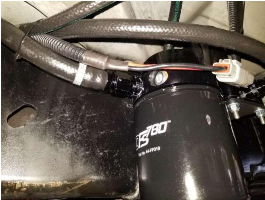
36. Plug the weatherproof connector on the end of the supplied power harness into the mating connector on the fuel manifold assembly motor.
