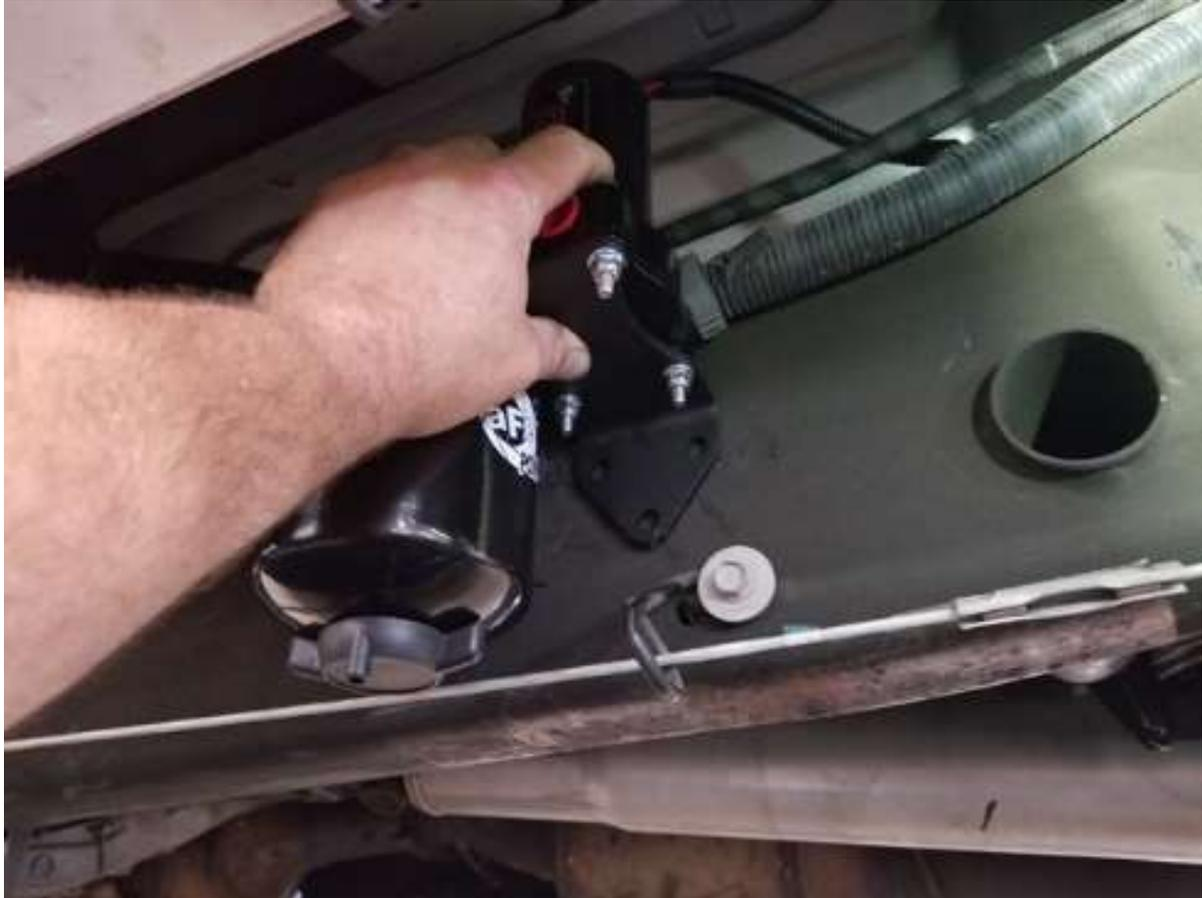
**23.** Place the fuel manifold assembly on to the truck and mark the three holes using the carbon steel frame bracket.
