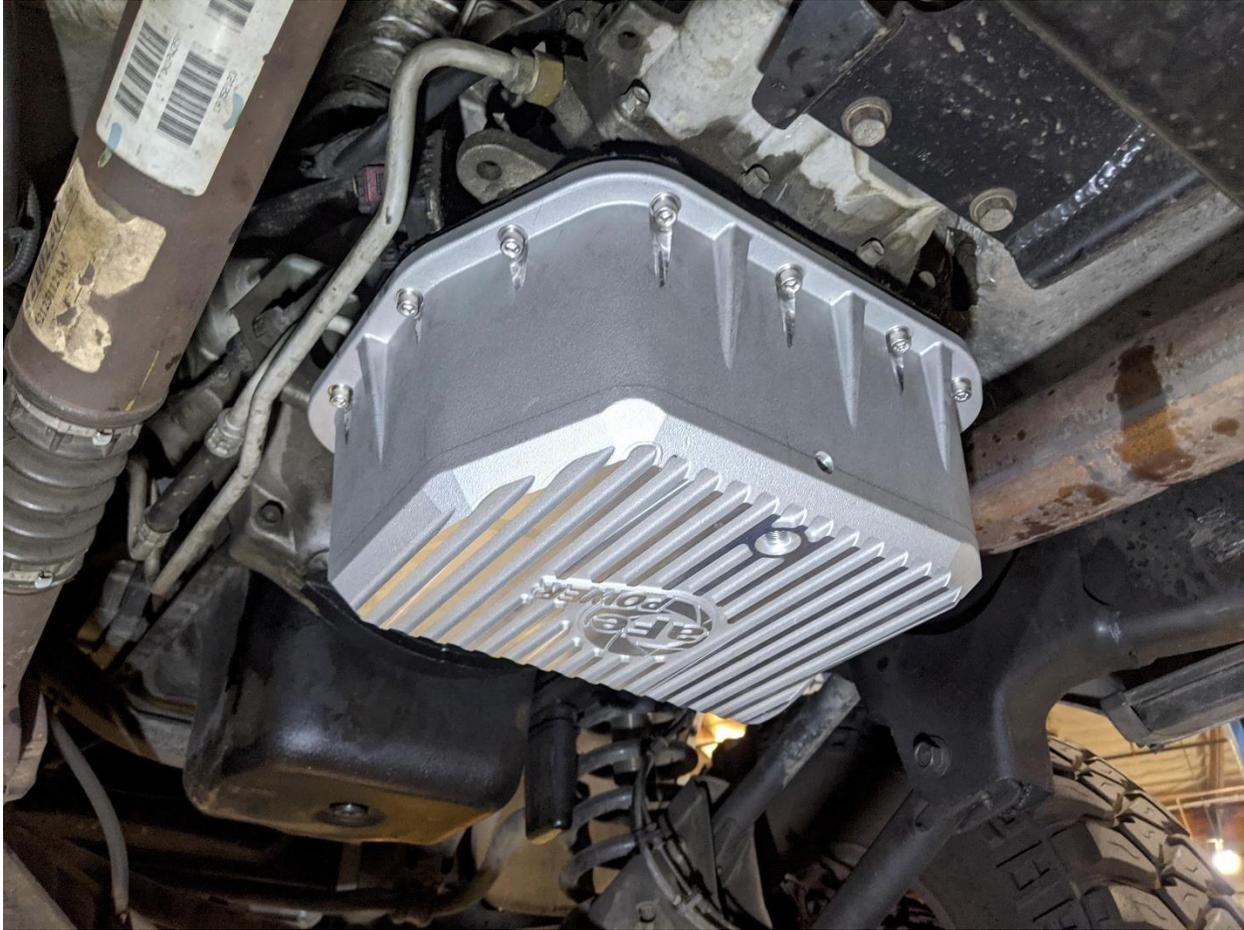
16. Hold the transmission pan up into position, aligning the screw holes. Install four (4) 5/16"-18 socket head screws and 5/16" flat washers into each of the corners to hold the pan into position.
