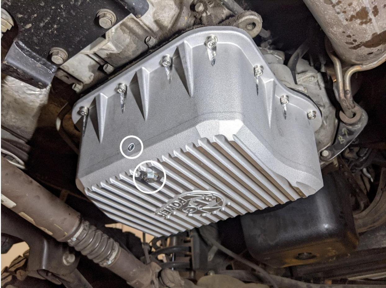
19. Install the supplied M12x1.25 magnetic drain plug and crush washer (secure about ½ turn past finger tight).
