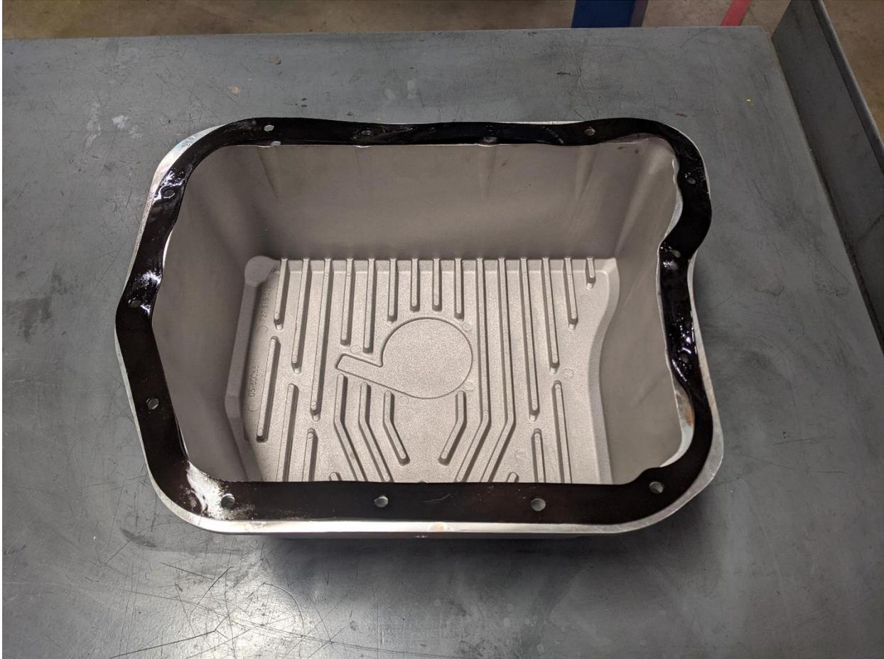
13. Hold the supplied aFe transmission pan up to the gasket surface to make sure you will be able to maneuver it into place.
