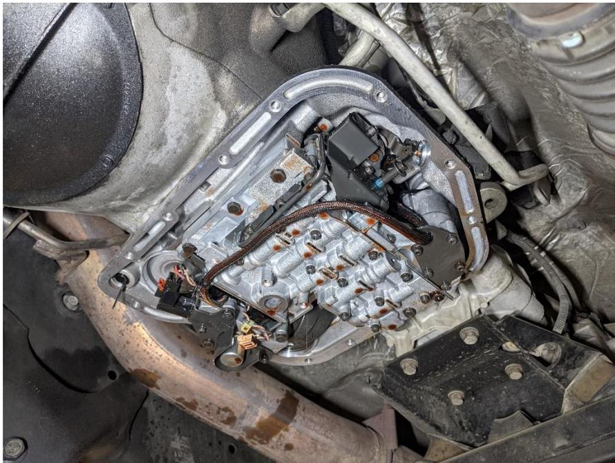
9. Clean the sealing surface with a gasket scraper. Be careful not to gouge the surface while cleaning.
