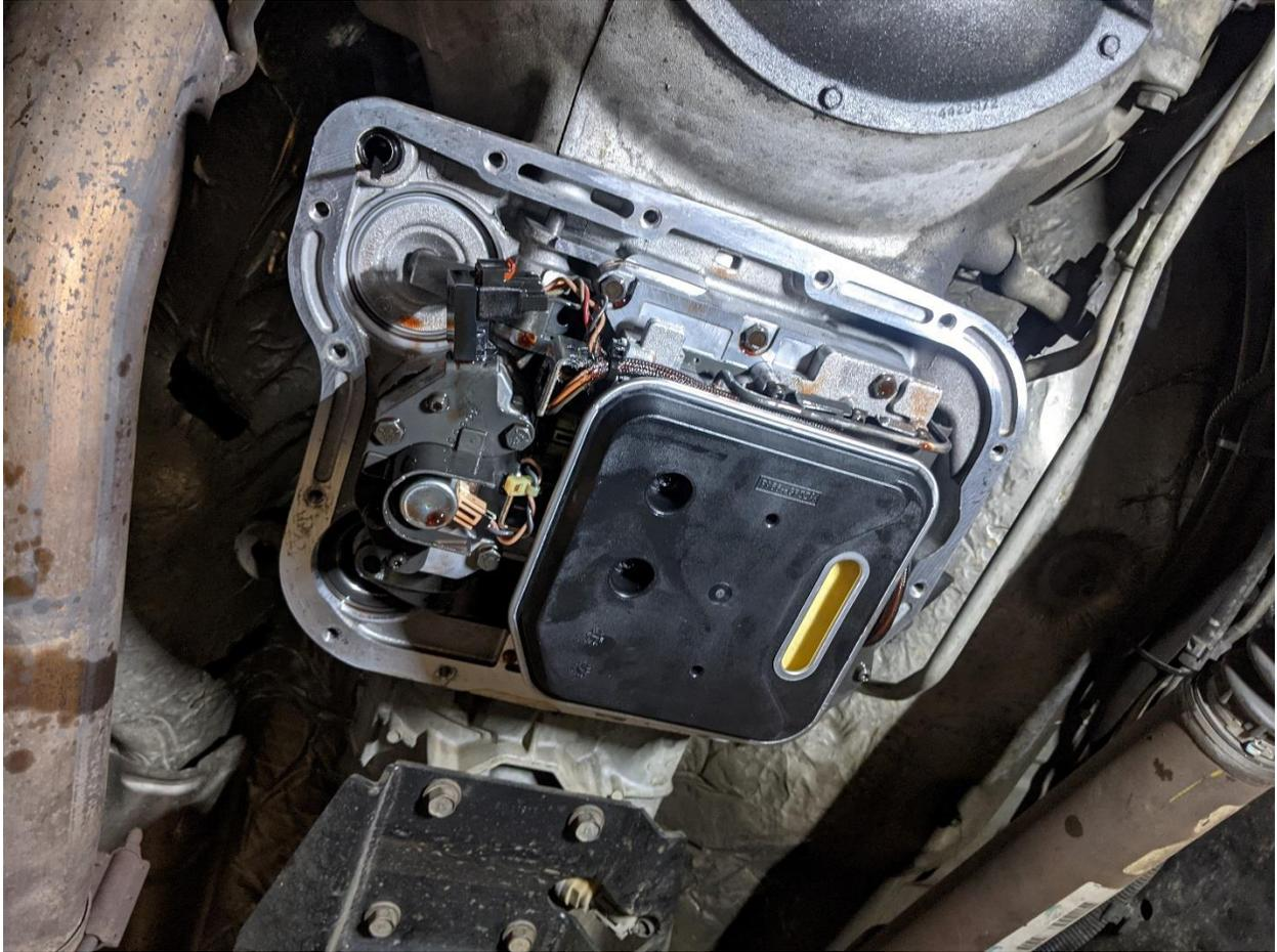
11. Allow the remaining oil in the casing to drain out until there are periodic drips.
