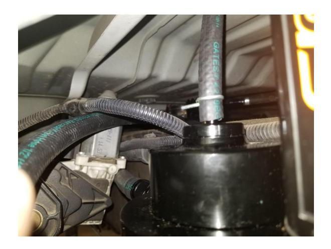
17. Carefully route the ¼" hose to the top of the air chamber on the fuel manifold assembly, making sure not to kink the hose or allow it near moving parts. Carefully mark and then cut the hose to the correct length. Using the supplied spring clamp, attach the hose to the nipple on the top of the air chamber on the fuel manifold assembly.
