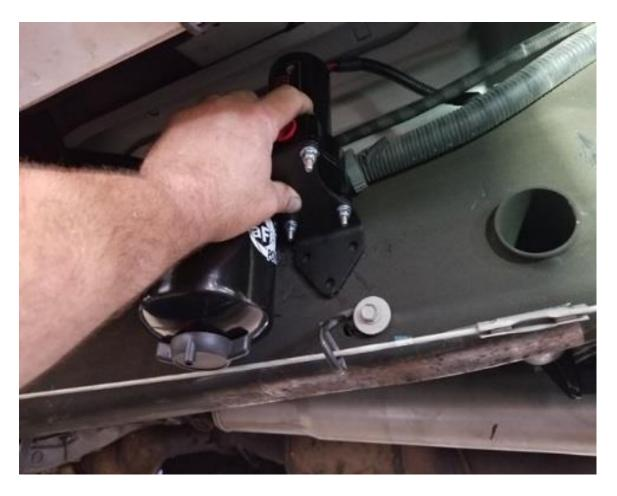
4. Place the fuel manifold assembly on to the truck and mark the three holes using the carbon steel frame bracket.
