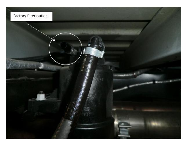
**Engine fuel supply line shown in Photo above.**
