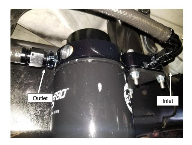
15. Attach the fittings to the inlet & outlet ports of the fuel manifold assembly. Make sure all connections are tight.
