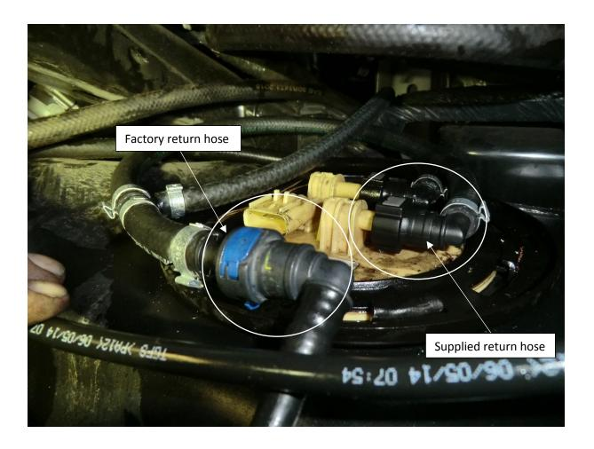
16. Disconnect the factory fuel return line on the top of the fuel tank. Attach the supplied fuel return hose between the male and female factory fuel fittings. Push all connections together.
