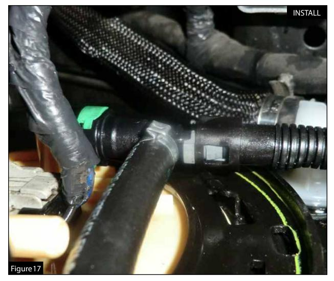
Step 21: Connect the factory fuel return line (female connection) onto the tee fitting at the end of the supplied fuel return line (male connection).
