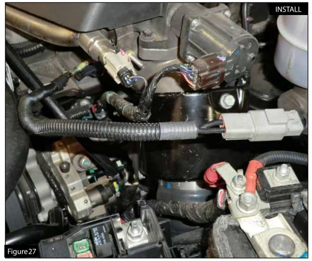
Step 35: Plug the supplied wire loom into the pressure sensor.
