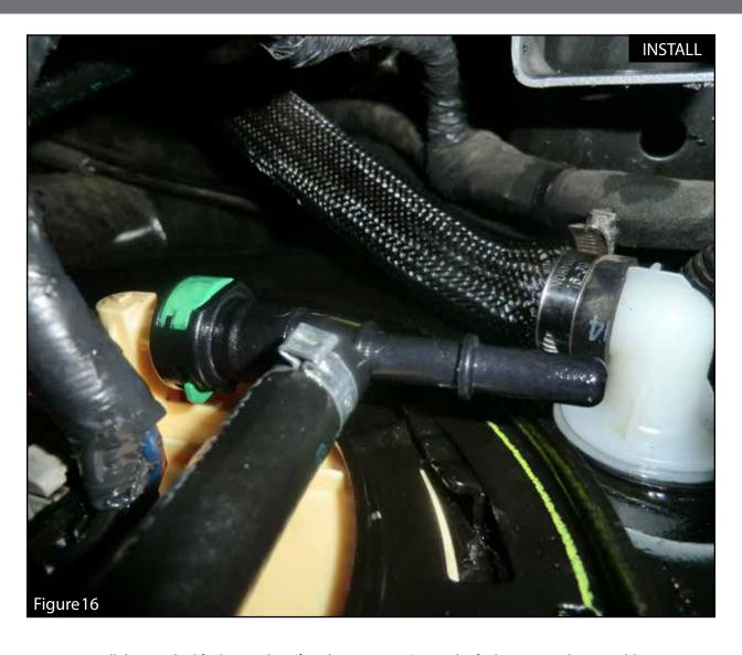
Step 19: Install the supplied fuel return line (female connection) onto the fuel pump sender assembly (male connection).
