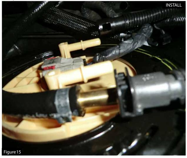
Step 18: Install the 3/8" quick disconnect fitting (male connection) on the supplied fuel outlet hose into the quick disconnect fitting (female connection) on the stock fuel feed line.
