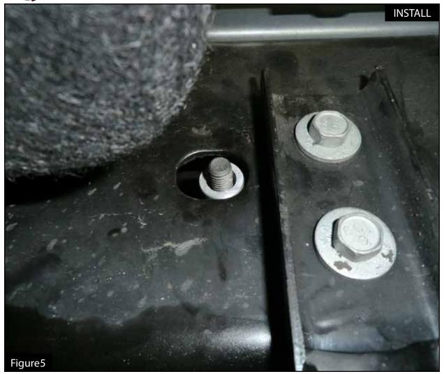
Step 6: Install the supplied aluminum spacer onto the 3/8" bolt.
