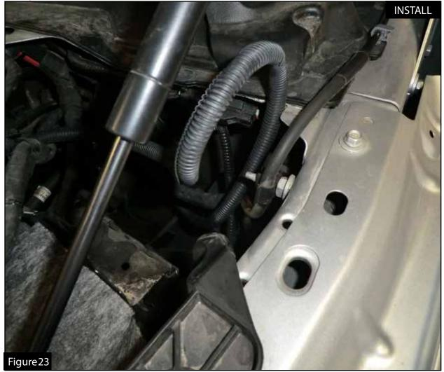
Step 31: Run the remaining wire harness along the frame to the engine compartment. Secure using supplied nylon cable ties.
