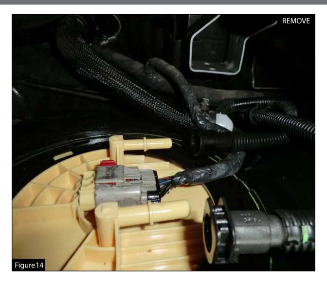
Step 15: Locate the factory fuel feed and return lines. They are located at the top of the fuel tank near the center of the tank.
