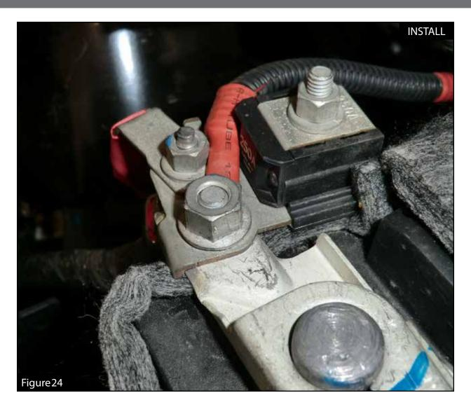
Step 32: Connect the red wire ring terminal to the positive side of the battery.
