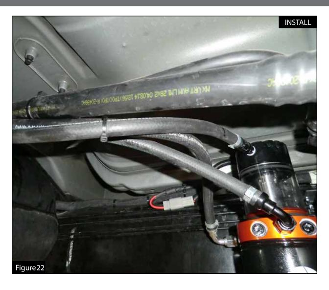
Step 29: Route the hoses as shown and secure with the supplied nylon cable ties.
