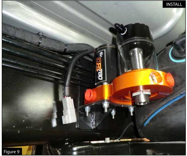
Step 10: Connect the DFS780 manifold to the bracket using the four (4) supplied M6 flange nuts (make sure the fiber washers isolate the pump body from the bracket).
