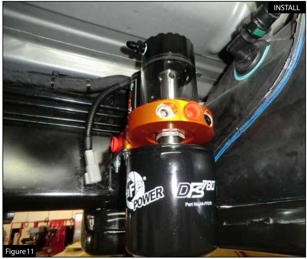
Step 12: Using a light oil, lube the gasket on the fuel filter before installation. Thread supplied water separator bowl onto the supplied fuel filter.
