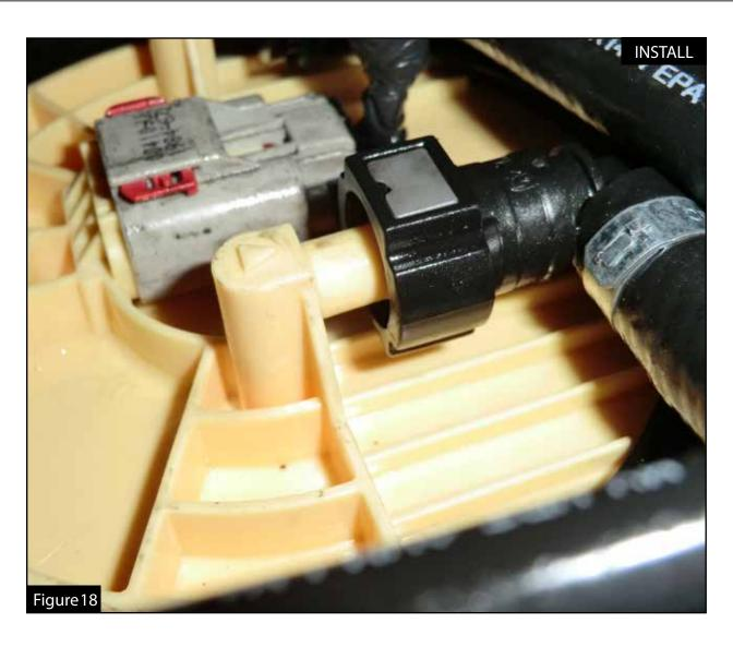
Step 22: Install the 90 degree 3/8" quick disconnect fitting (female connection) on the supplied fuel inlet hose onto the quick disconnect fitting (male connection) on the fuel pump sender assembly.
