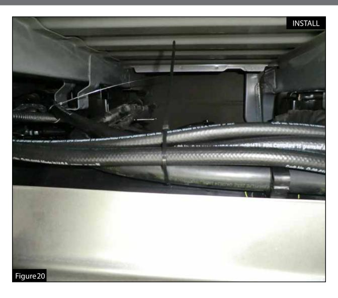
Step 25: Route the hoses as shown and secure with the supplied nylon cable ties.
