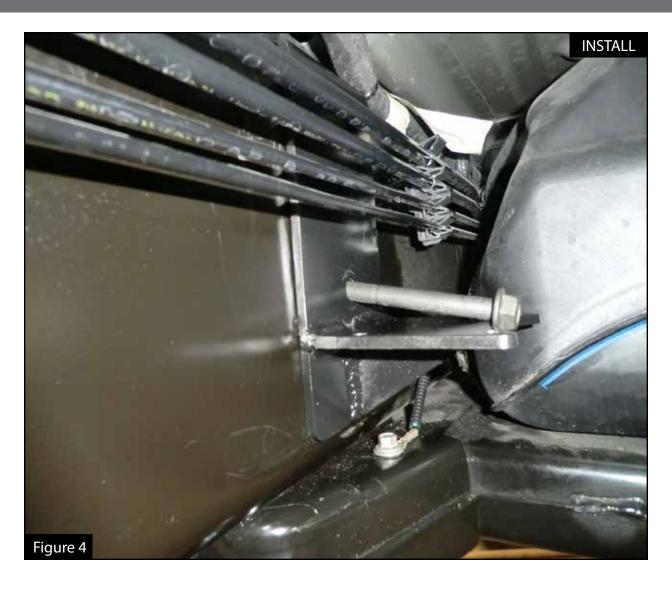
Step 5: Install the supplied 3/8" bolt into the bracket and through the frame rail.
