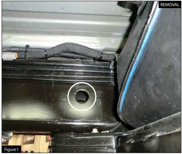
Step 1: Locate the hole in the driver's side frame rail behind the DEF tank and in front of the fuel tank.
