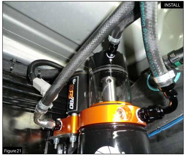
Step 26: Install the supplied inlet fuel line (90° silver "AN" fitting) onto the fuel inlet port of the DFS780 manifold.
