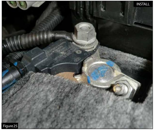
Step 33: Connect the black wire ring terminal to the negative side on the battery.
