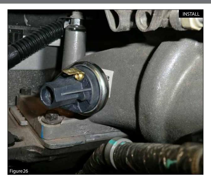
Step 34: Install the supplied pressure sensor into the intake manifold (1/8" NPT).
