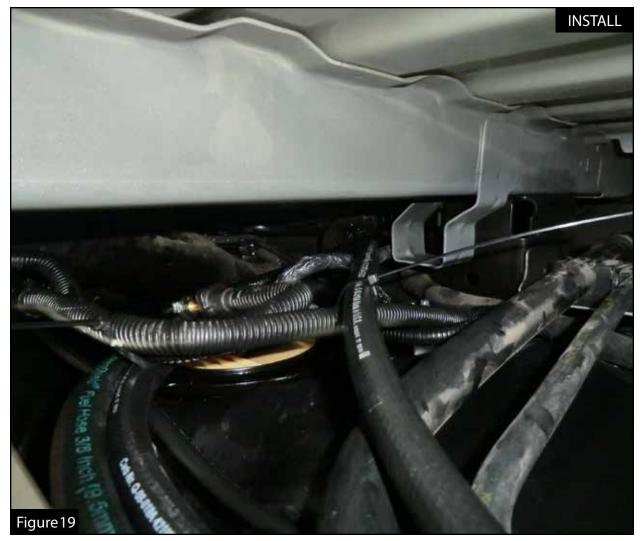
Step 24: Route the hoses as shown and secure with the supplied nylon cable ties.
