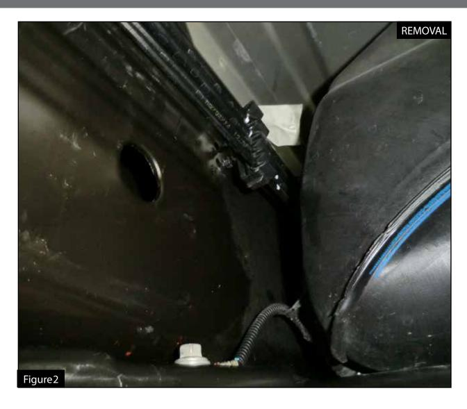
Step 2: Gently pull the hard lines off of the frame rail. Be careful not to bend or kink the hard lines.
