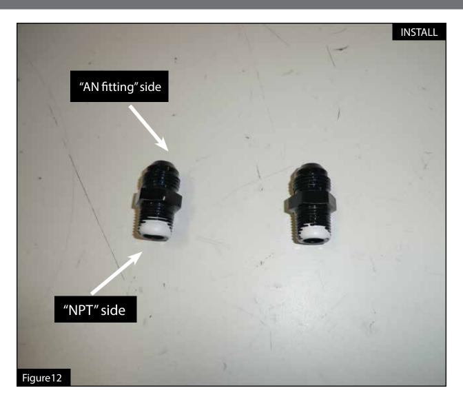
Step 13: Apply Teflon tape (PTFE) or Teflon paste (PTFE) to the  $2 \times 3/8$ " NPT to -6 AN fittings.
