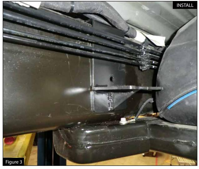
Step 3: Place the supplied bracket between the frame and the hard lines.
