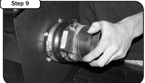
Step 9 Slide the MAF sensor, clamps (#072 and #064), and reducer coupler (05-00020) on the air filter adaptor. Do not tighten the clamps at this time.
