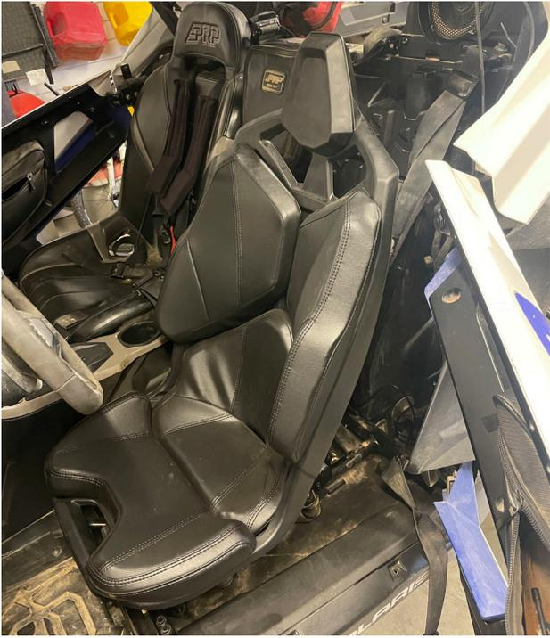
**1. Start by Removing the stock seats from the vehicle. Slide it all the way forward, and pull the release lever.**
