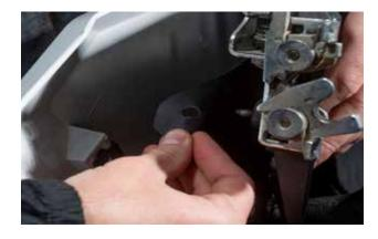
Line up the cut-holes on the bags liner, with the corresponding bolt holes on the frame and plastic panel. Re-install the bolts so that the bag is secured between the door's frame and plastic panel.
