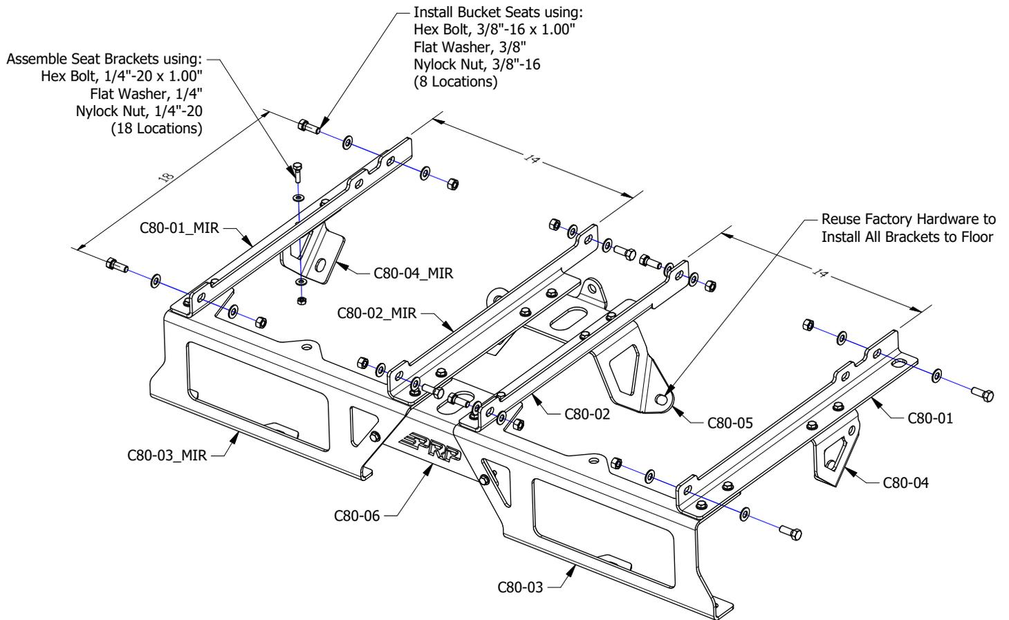
7a) Install the PRP Seats by lining up the tabs on the seats to the holes on the angle brackets. Use the supplied 3/8"-16 x 1" bolts, nuts, and washers.
