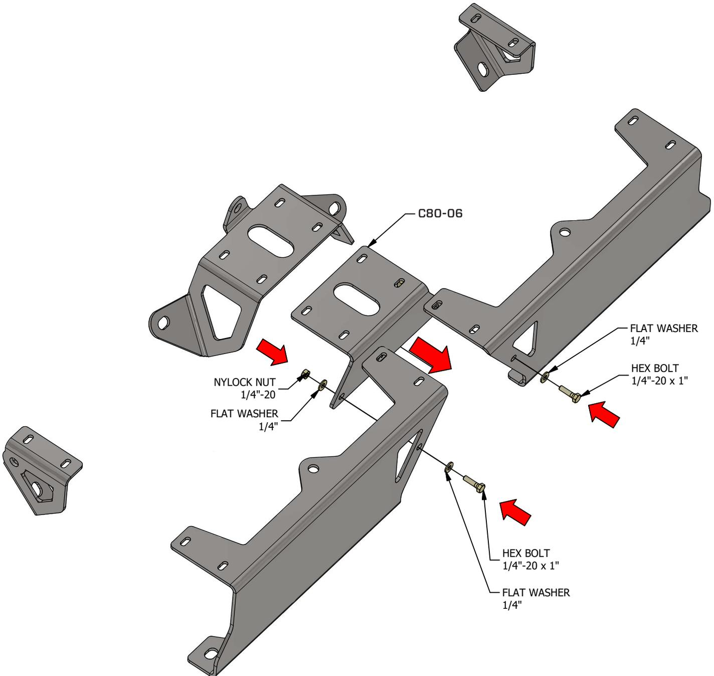
4) Install the C80-06 Center PRP Bracket using the supplied hardware.
