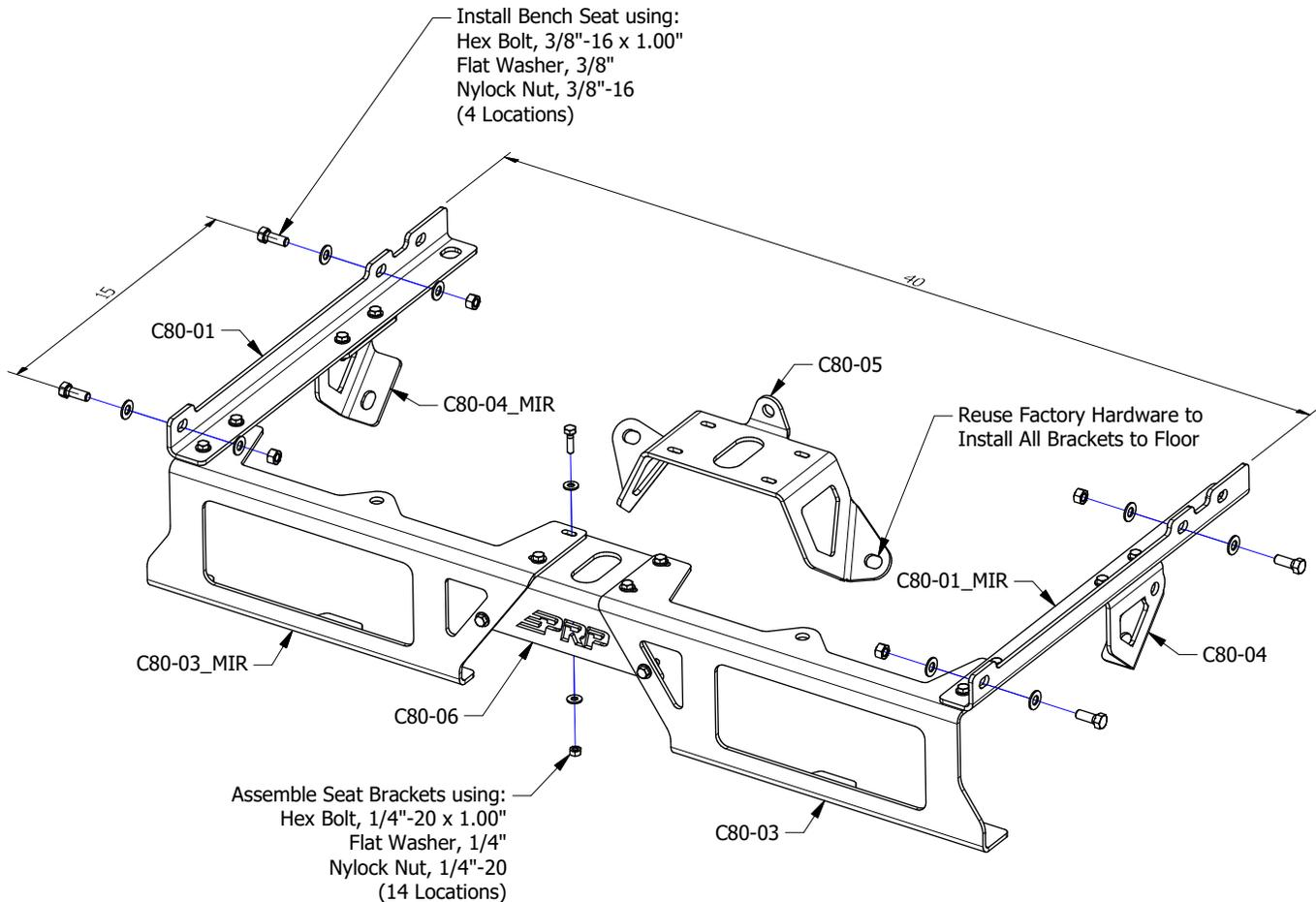
7b) Install the PRP Bench by lining up the tabs on the bench to the holes on the angle brackets. Use the supplied 3/8"-16 x 1" bolts, nuts, and washers.
