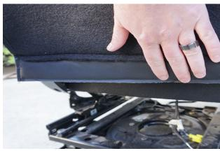
**8.** Remove the felt strips covering the hook&loop strips, then connect the back flap of the cover to the center flap that you just pushed through. Try to get these as tight as possible to ensure a tight fitting cover.
