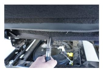
12. Pull the rest of the bottom cover back and start to attach it to the seat. Push the side edges of the cover down and underneath the plastic trim.
