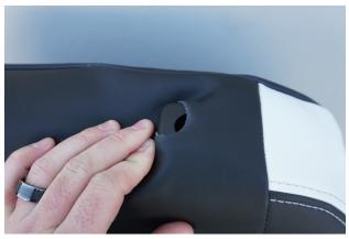
**5.** On the top of the seat, you will need to push the plastic headrest slots through the holes in the cover. Push one corner of the hole underneath the plastic, then work your way around and push the cover under the other 3 corners until the plastic sits flush on top of the cover.
