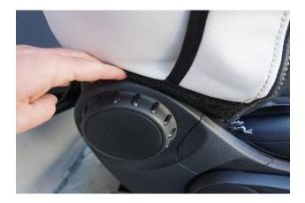
**6.** On the sides of the seat, push the cover under/behind the seat plastic seat adjusters to that the cover material sits flat and isnt bunched up.
