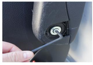
3. Next remove the armrest on the side of the seat. Use a Flat Head Screwdriver to remove the plastic cover. Then use a 5mm Allen wrench to remove the bolt, and pull off the armrest. (This may take some force to do as the armrests tend to get tweaked over time and use).
