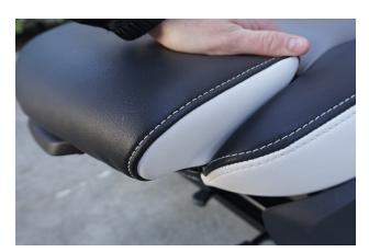
**9.** The airbag slot on the shoulder has a mesh liner that needs to be tucked underneath the vinyl, so that it sits flat on the front of the seat. Start at the top, and use your hands to tuck this mesh into & under the cover.
