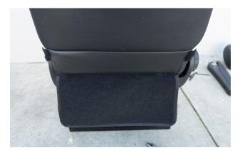
**18.** On the back of the seat, let the carpet flap come down, and then use the elastic band to connect it underneath the seat. That way the carpet flap stays tucked up and out of the way.
