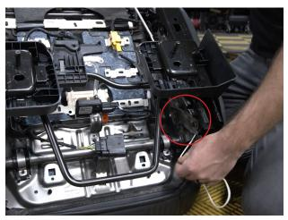
10. Under the seat, you will run the draw string on the door side behind these two metal lift brackets above the slider, and then feed it into the ribbon loop on the back flap of our cover.
