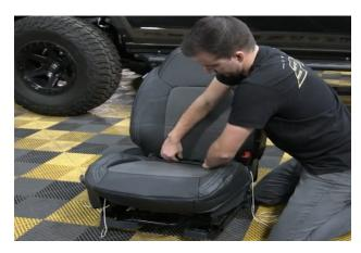
5. Remove headrest and slide the top of the front cover over the top. Pull it down over the seat, and tuck in the corners of the cover around the plastic lever. Play with the cover and move it around until it fits nice.
