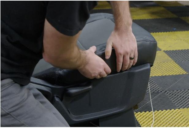
9. On the side of the seat, take the section with no draw string, and tuck it under the plastic skirt of the side of the seat. \*You can do this with your fingers or use a flat blade tucking tool.
