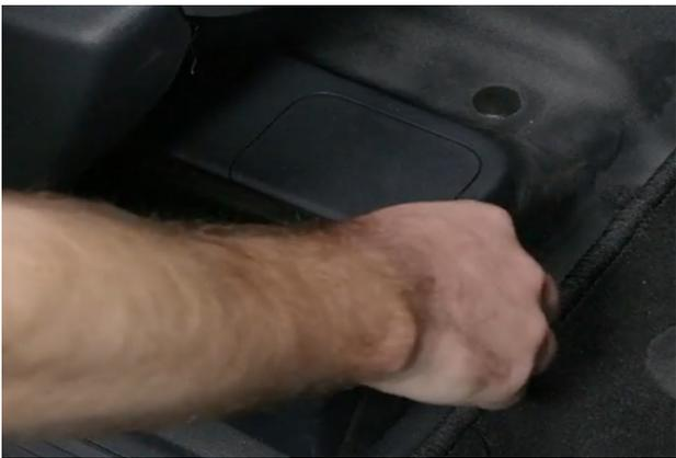
2. To remove the seat - Slide the seat back to reveal the two plastic covers at the front of the seat.
