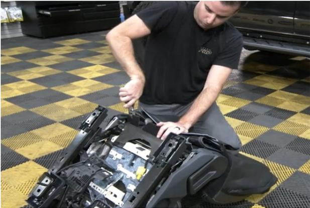
6. Take the flap on the front cover and slide it through the seat in the crevice between the bottom and back of the seat.
