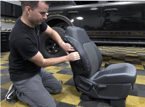
7. The airbag slot on the shoulder has a mesh liner that needs to be tucked underneath the vinyl, so that it sits flat on the front of the seat. Start at the top, and use your hands to tuck this mesh into & under the cover.
