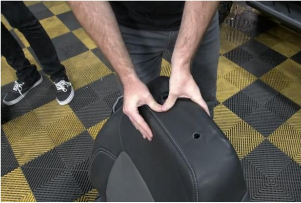
5. Remove headrest and slide the top of the front cover over the top. Pull it down over the seat, and tuck in the corners of the cover around the plastic lever. Play with the cover and move it around until it fits nice.
