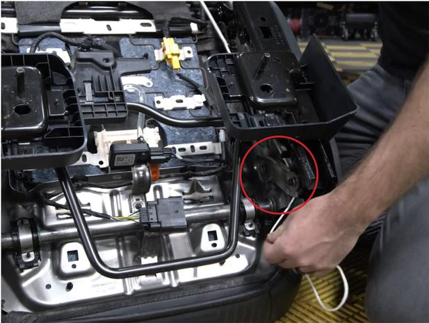
10. Under the seat, you will run the draw string on the door side behind these two metal lift brackets above the slider, and then feed it into the ribbon loop on the back flap of our cover.
