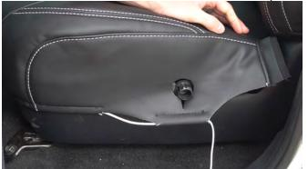
9. Tuck the cover under the Adjustment Levers
