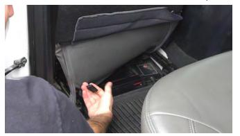
The top portion of the OEM cover has a flap that wraps around the back & bottom of the seat - Blocking access to the flap you just pushed through.
