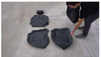
Place the covers out in the sun. This will allow the material to warm up and get rid of most creases formed from being in the box. This also makes it easier to fit the covers over the seat.
