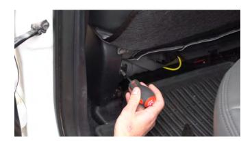
10b. Tuck the edges underneath the side skirt Option 2 - We found it much easier to remove this plastic skirt entirely to install. Use a Phillips head screwdriver to remove the screw on the back of the seat. Then pull the plastic skirt off and slide it forward. There is a push-pin in the center of the plastic, then a sliding bracket in the front that requires you to slide the skirt forward to release.
