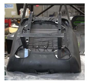
12. Now that the assembly is complete, place the seat back into the vehicle. Make sure that the front bar on the seat base is lined up correctly into the bracket on the floor, and that plastic release handle on the rear of the seat clicks and locks into place.
