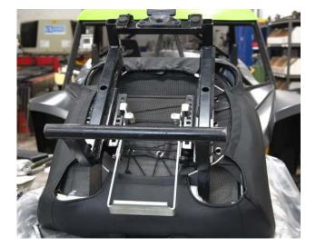
Then place the supplied Square Tube on top of each parallel bar, with the bolt holes lined up. Use the supplied hardware: 4x 3/16" Allen head bolts, 8x washers, and 4x 7/16" nuts to attach each square tube bracket and release handle bracket to the bottom of the seat. Tighten down all 4 bolts/nuts using a 3/16" Allen and 7/16" wrench. [Torgue to 144 in-lbs].
