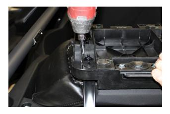
2. Using a #4 Allen remove the four bolts holding the plastic pan to the stock seat.
