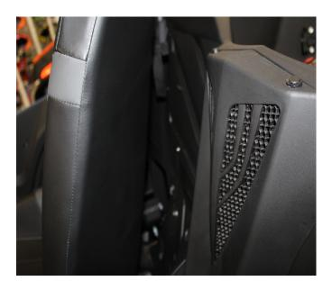
6. (Optional) Once the PRP seat is installed you will notice that is wider than your stock seat and hits the inside plastic panel. If you want the seat to slide back farther, you will have to trim this plastic piece. PRP does not have instructions on how or where to do this.
