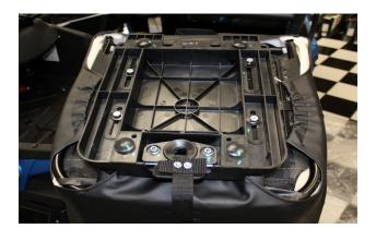
3. Turn the PRP seat upside down on its head and place the plastic pan onto the PRP Seat.
