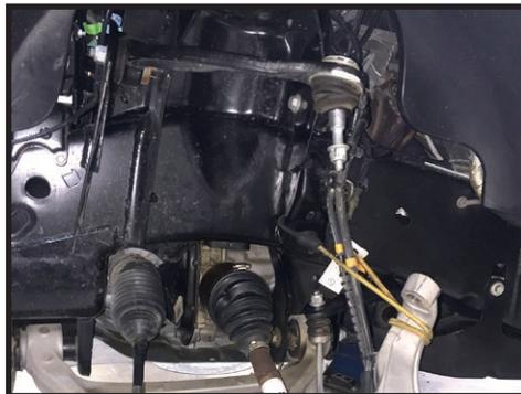
4. Follow the Live Valve back to the connector then disconnect the Live Valve and wire retainers. [FIGURE 2 & 3]
