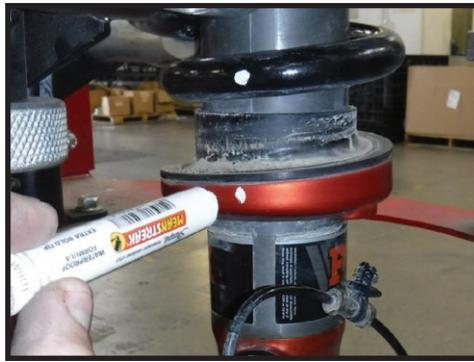
7. It is not necessary to disassemble the shock or coil, however the spring will need to be compressed a couple of inches. A quality spring compressor is necessary; we recommend a three arm style as shown in the photos. [FIGURE 5 & 6]
