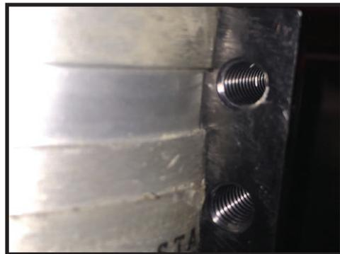
**10.** As you release tension make sure you have maintained alignment with your marks. By putting a rod or extension in the lower eyelet you can visually check that it is in line with the 3rd mount bolt. [FIGURE 15]
