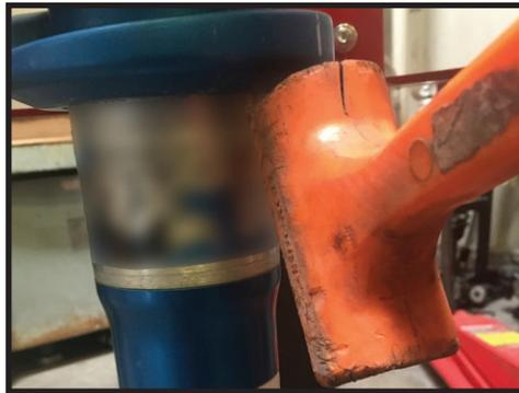
**9.** Position the split preload collar on the shock with the text of the desired lift height right side up (note the lift height indicated assumes the upper shim ring is also used). The bolt heads of the collar should be towards the live valve actuator [Tighten bolts to 12 ft-lbs]. Make sure that the inner locking portion of the collar is securely seated inside the groove on the shock body. [FIGURE 14]
