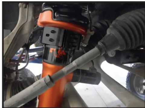
**11.** Reinstall in vehicle: slide the upper 3/8\"/>
