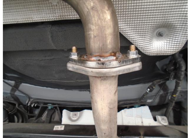
**Step 2:** Begin Installing the new MagnaFlow system by attaching the inlet pipe to the OE outlet using the supplied fasteners and gasket.
