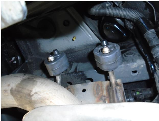
**Step 1:** To remove the OE muffler assembly unfasten the hardware at the flange. While supporting the muffler extract the hangers from the rubber insulators (retain rubber insulators as they will be re-used).
