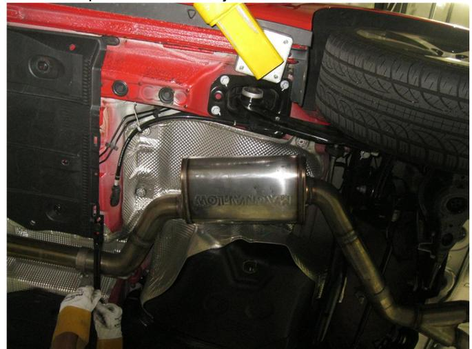
**Step 3.** Next attach the Muffler Assembly to the Inlet Pipe using the supplied 3.00" clamp and by fitting the hangers into the rubber insulators. Use the supplied Rubber Insulator for the welded hanger rearward of the muffler if applicable.
