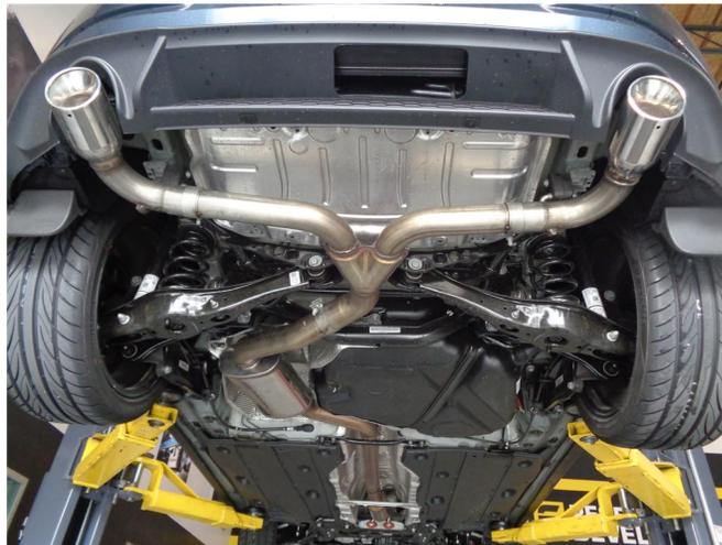
**Step 4.** Next attach the Y-Pipe Assembly to the Muffler Assembly using the supplied 3.00" clamp. Install the two Tail Pipe Assemblies in a similar fashion using the supplied 2.50" clamps. Locate the welded hangers to the rubber insulators.
