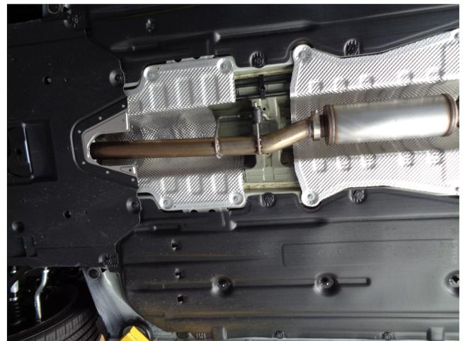
Step 3: Next loosely fasten the Resonator Assembly to the Inlet pipe using the supplied clamp.
