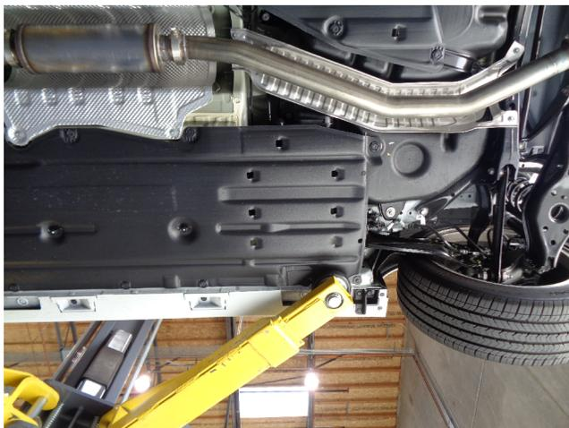
Step 3: Next attach the Mid Extension Pipe to the Resonator Assembly using the supplied clamp.
