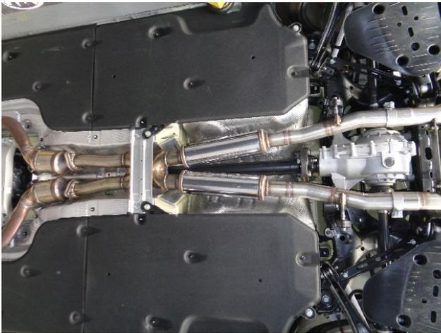
**Step 2:** Begin installation of the new system by fastening the Resonator Assembly inlets to the catalytic converter using the OEM fasteners (Leave all clamps and fasteners loose for final adjustment of the complete system.)
