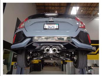
**Step 5:** Once a final position has been chosen for the new exhaust system, evenly tingten all clamps from front to rear using the torque specifications on page one of these instructions. Inspect all fasteners after 25-50 miles for operation and re-tighten if necessary.
