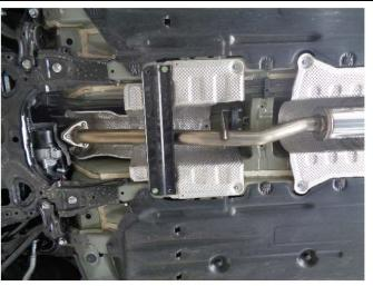
**Step 2:** Begin installing your new system by loosely bolting both inlet flange of the Resonator Assemblies to the catalytic converter outlets using the OEM hardware. Engage the welded hangers to the rubber insulator.
