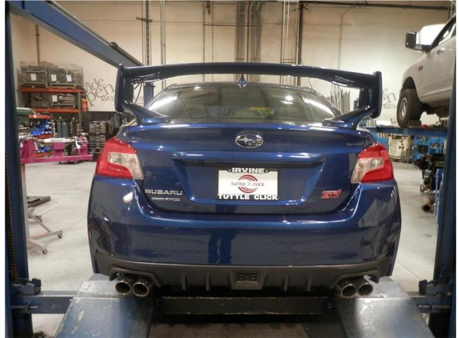
**Step 3.** Once a final position has been chosen for the new system, evenly tighten all clamps from front to rear using the torque specifications on page one of the instructions. Inspect all fasteners after 25-50 miles of operation and re-tighten if necessary.
