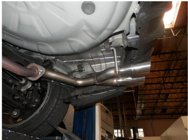
**Step 2.** Next loosely install both Tail Pipes by bolting the inlets flanges to the Y-Pipe Assembly using the OEM hardware. Insert all welded hangers into the OEM rubber insulators.
