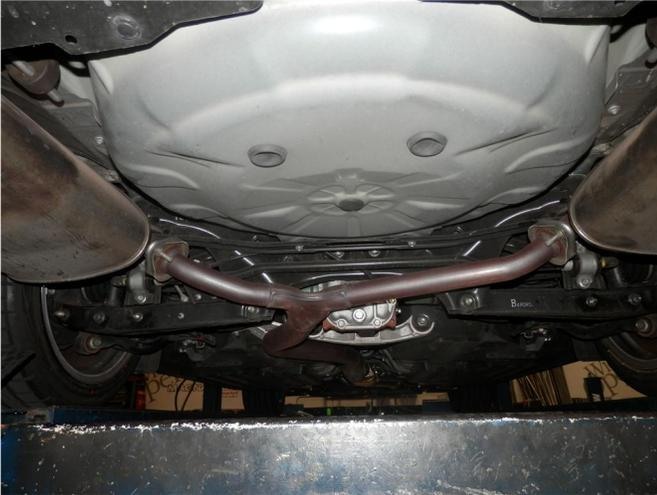
**Step 1.** Remove both muffer assemblies by unbolting them from OEM Y-Pipe assembly. Remove all welded hangers from the rubber insulators. The exhaust system may now be removed. Retain all mounting hardware as it will be needed to install your new MAGNAFLOW system.
