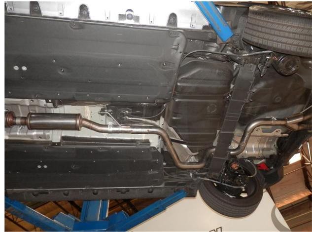
**Step 3.** Next, install the Mid Pipe Assembly, the Tail Pipe Assembly using the supplied 2.50" clamps. Locate the welded hangers to the rubber insulators.
