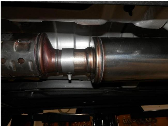
**Step 2.** Begin installation of your new MAGNAFLOW system by slipping the Resonator Assembly inlet end over the Catalytic Converter outlet. Loosely secure using the supplied 2.36" clamp. Leave all clamps loose during initial installation.
