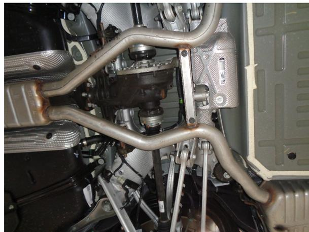
**Step 1.** To remove the OEM exhaust system, You can then disengage the welded hangers from the rubber insulators and remove the tailpipe assy. Unfasten the two brackets by the tailpipes, the clamp attaching the OEM inlet pipe assembly to the catalytic converter and the flange on the otherside. Do not damage or discard the inlet pipe clamp or rubber insulators as they will be re-used to mount the new system. Disengage the inlet pipe assembly hanger and remove the exhaust from the vehicle.
