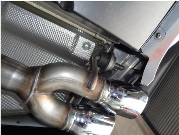
**Step 3.** Using the supplied rubber insulators install the Tailpipe Assemblies to the Muffler fitting the hangers into the installed hanger brackets. Install the bracket in between the two tailpipes.
