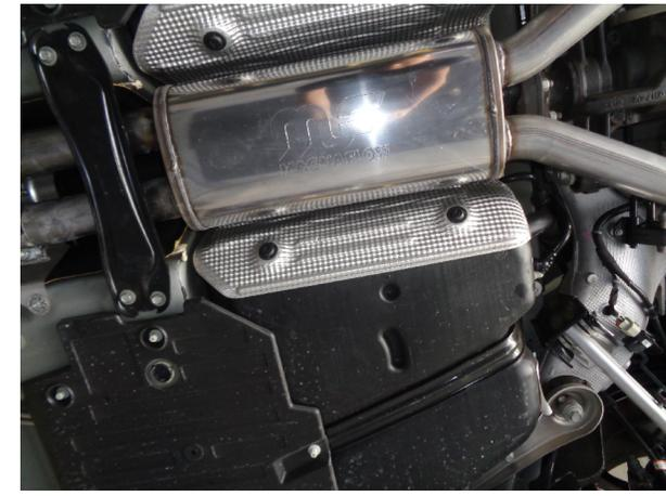
**Step 2.** To begin, fasten the Inlet pipe assembly to the outlet of the OE system using the OE clamp assembly and by fitting the welded hanger into the rubber insulator (Leave all clamps and fasteners loose for final adjustment of the complete system.)
