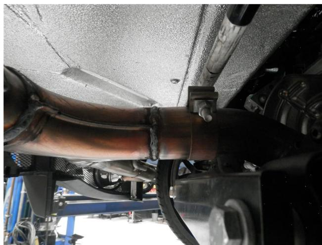
**Step 3.** Next loosely attach the Tail Pipe Assembly to the Inlet Pipe Assembly using the supplied 2.50" clamps. Engage all welded hangers to the rubber insulators.
