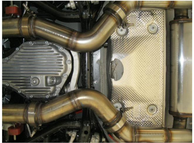
**Step 4.** Loosely Install the D/S and P/S Mid Pipe Assemblies with the supplied V-Band Clamps.
