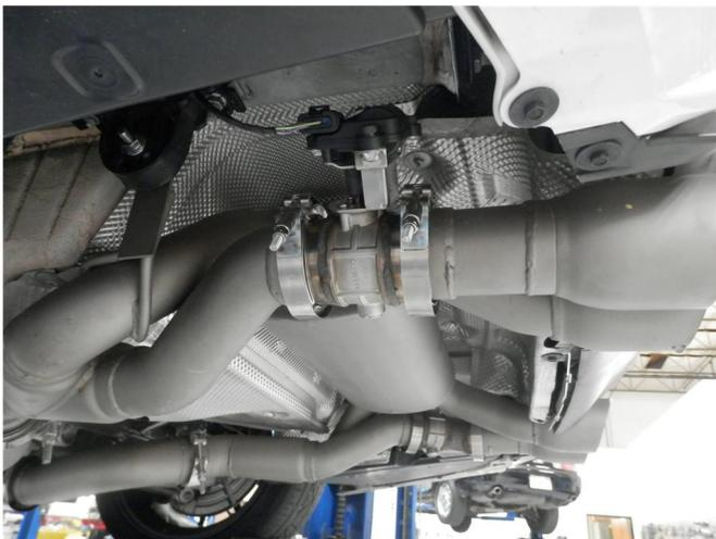
**Step 6.** Re-attach the electrical plugs to each valve motor.
