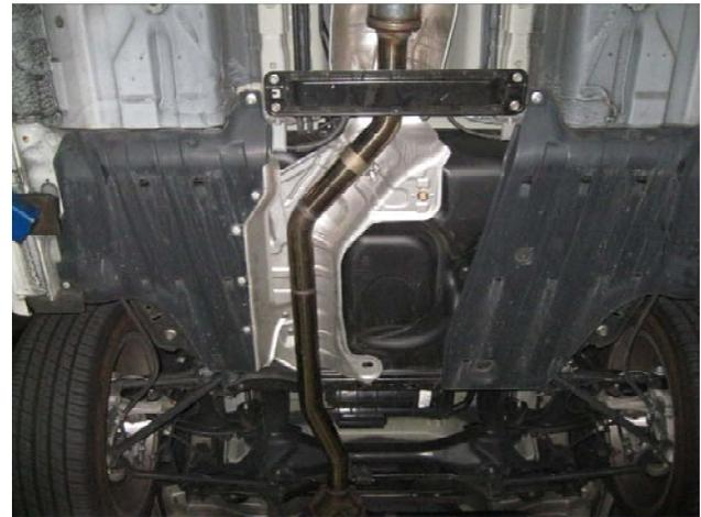
**Step 3.** Next use the supplied 2.25" clamp to attach the Y-Pipe Assembly to the Resonator Assembly and insert the hanger to rubber insulator.
