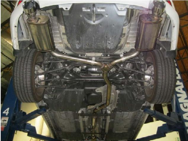
**Step 4.** Next use the supplied 2.25" clamps to attach the Muffler Assemblies to the Y-Pipe Assembly and insert the hangers into rubber insulators.
