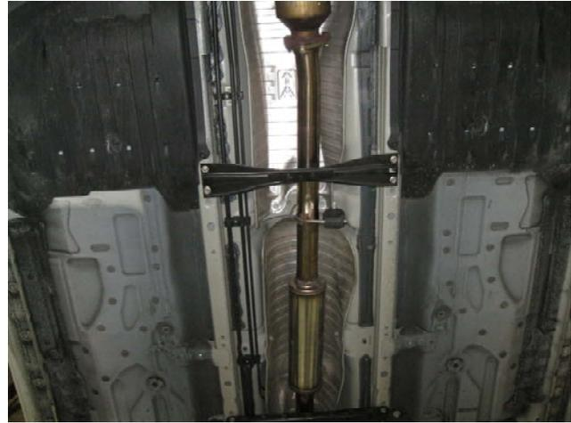
**Step 2.** Begin installation of your new MAGNAFLOW system by attaching the Resonator Assembly to the catalytic converter outlet using the OEM fasteners and insulator. Keep all fasteners and clamps loose until final adjustment.
