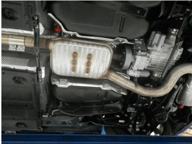
**Step 2.** Begin removal of the OEM system by loosening the slip clamp at the vehicles exhaust inlet. Working front to rear disengage all welded hangers from the rubber insulators. Be sure to retain all mounting hardware as it will be needed to mount your new MAGNAFLOW exhaust.
