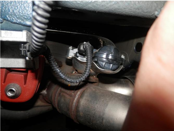
**Step 1.** Before removing the OEM exhaust system you will need to unplug the electrical connectors for both exhaust control valves. These are located on the vehicles tail pipes.
