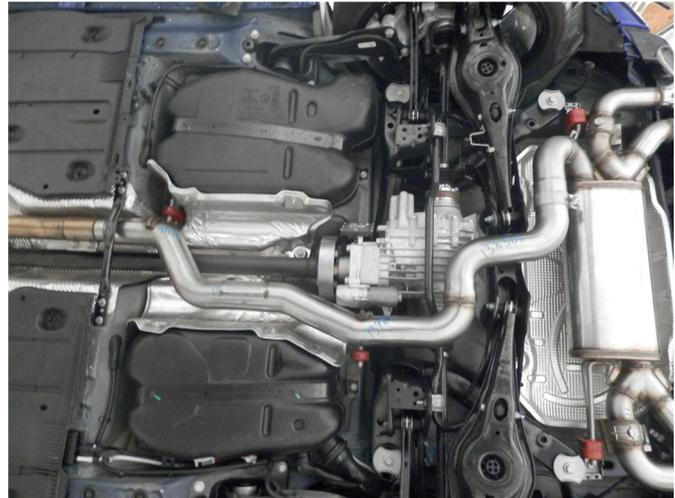
**Step 5.** Loosely attach the Inlet Pipe Assembly to the OEM slip clamp. Engage the welded hangers to the rubber insulators.
