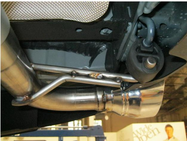
**Step 4.** Finish by installing both the Muffler Assembly and both Tip Assemblies using the supplied 250" clamps, fitting the hangers into the rubber insulators.
