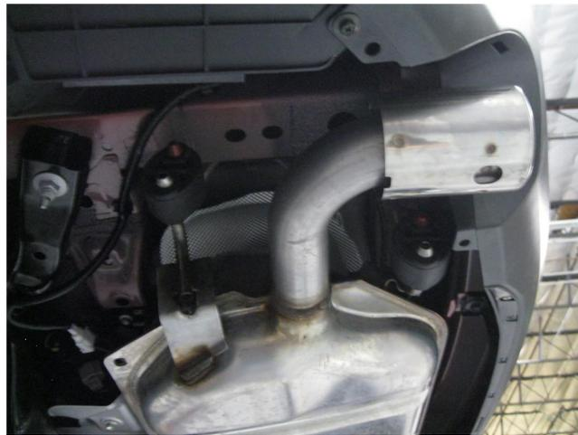
**Step 2.** Next, unbolt the flange at the muffler assembly inlet, disengage the hangers from the rubber insulators (save the rubber insulators as they will be used to install the new system) and remove the OEM system.
