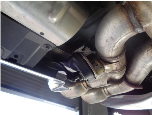
Step 2: Next you will need to unplug the electrical connection on the Exhaust Valve Control Motors (Qty 2) located on the OEM exhaust assembly.
