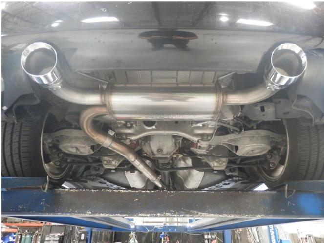
**Step 5.** Loosely attach the Muffler Assembly to the Mid Pipe Assembly using the supplied clamp. Engage all welded hangers to the rubber insulators.
