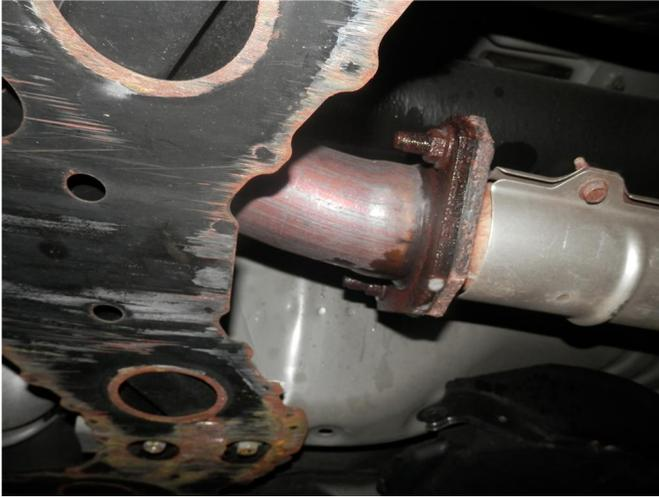
**Step 1.** Begin removal of the OEM exhaust system by unbolting the flanges attaching the exhaust to the catalytic converter. Do not discard or damage the OEM fasteners or rubber insulators as they will be used to install the new system.
