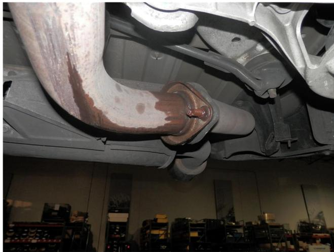
**Step 2.** Unbolt the flange junction between the mid pipe and the muffler assembly. Unfasten the ground strap from the muffler (this will not be re-attached) and disengage the hangers from rubber insulators. You can now remove the OEM exhaust.
