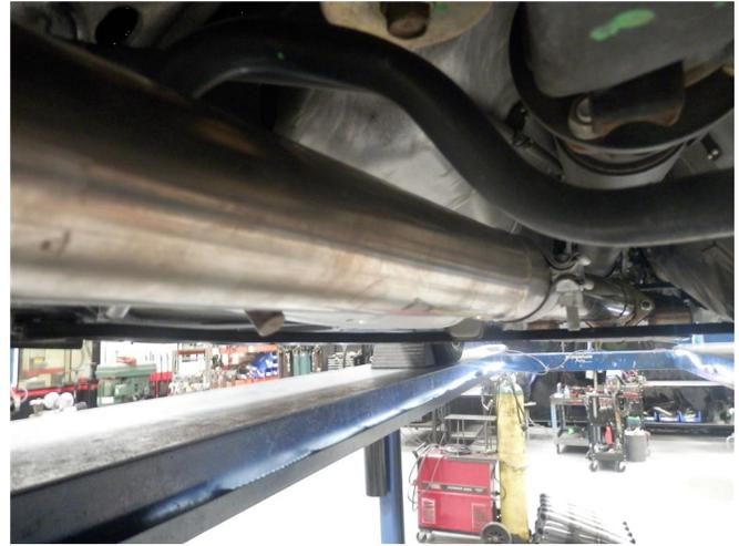
**Step 3.** Begin installation of your new MAGNAFLOW system by attaching the flanges of the Inlet Pipe Assembly to the catalytic converter outlet using the OEM hardware. Keep all fasteners and clamps loose until final adjustment.
