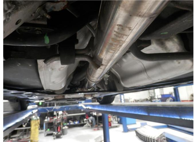
**Step 4.** Next loosely attach the Mid Pipe Assembly to the Inlet Pipe Assembly using the supplied clamp. Engage the welded hanger to the rubber insulator.
