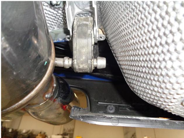
**Step 3.** Next, install the Mid Pipes to the Resonator Assembly using the supplied 2.25" clamps. Finish by attaching the Muffler Assemblies to the Mid Pipes using the supplied 2.25" clamps. Insert hangers into rubber insulators.
