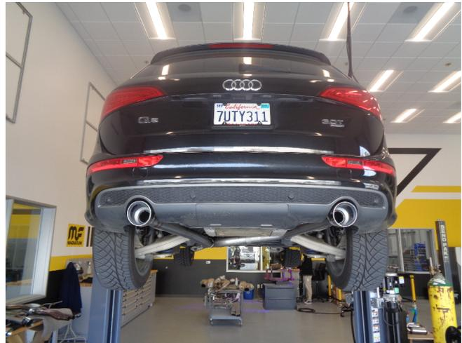
Step 4: Once a final position has been chosen for the new exhaust system, evenly tighten all clamps from front to rear using the torque specifications on page one of these instructions. Inspect all fasteners after 25-50 miles for operation and re-tighten if necessary.
