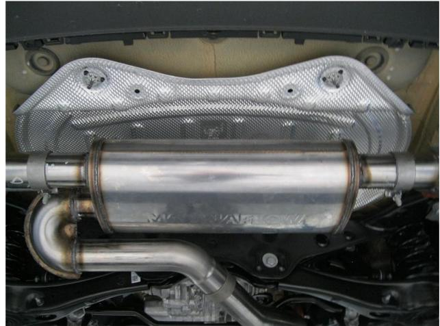
**Step 3.** Next Install the Muffer Assembly using the supplied 2.50" clamp and fit the welded hanger into the rubber insulator.
