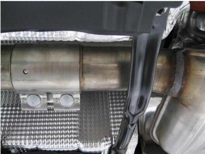
**Step 2.** Begin installation of the new system by attaching the Inlet Pipe Assembly to the factory outlet using the OEM clamp and fit the hangers into the rubber insulators. Leave all clamps loose until final adjustment.
