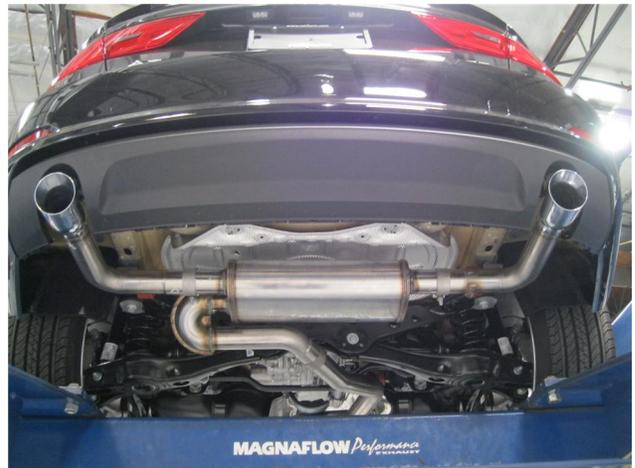
**Step 4.** Complete the installation by fastening the Driver and Passenger side Tailpipe Assemblies to the Muffer Assembly with the supplied 2.50" clamps and fit the hangers into the insulators. Re-install the factory brace.
