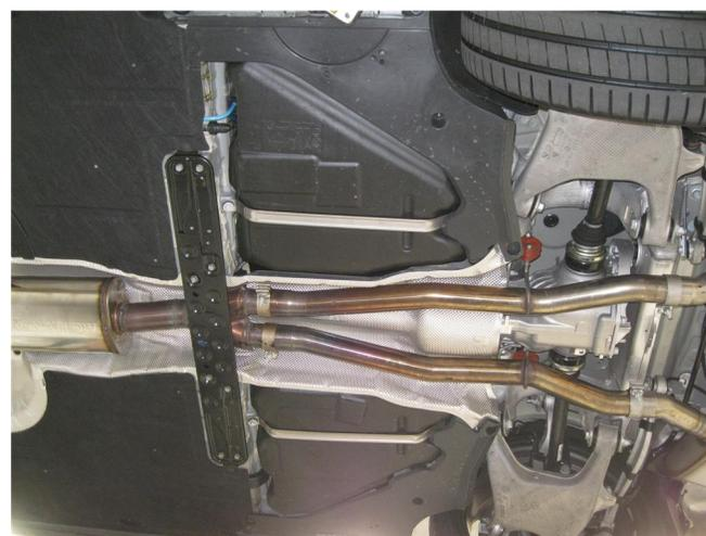
**Step 3.** Next attach the Resonator Assembly to the Y-Pipe Assembly followed by the two Mid-Pipe assemblies, use supplied clamps and fit hangers into rubber insulators.
