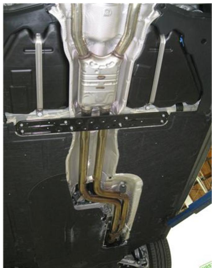
**Step 1. NOTICE;** to fit this exhaust system the vehicle must have a BMW M5 rear valance (P/N 51128050480) installed. To allow for extraction of the OEM system you must first remove the underside cross brace. Next loosen the clamp at the outlet of the catalytic converter. Working front to rear detach all hangers from rubber insulators and remove the system. Retain rubber insulators and clamp as they will be re-used the mount the new system.
