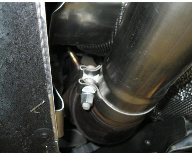
**Step 2.** Begin installation of the new system by fastening the Inlet Pipe to the outlet of the catalytic converter using the supplied 3.00" clamp.
