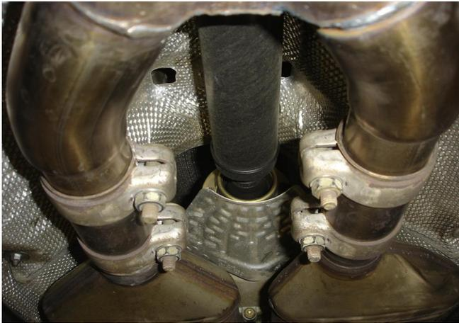
**Step 2.** Begin installation of your new exhaust system by inserting the inlet pipes of the X-Pipe Assembly into the two clamps at the catalytic converters locate the two welded hangers in the rubber insulators (leave all clamps loose for final adjustment of the complete system).
