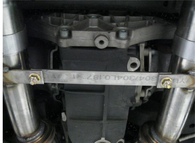
**Step 3.** Next Install the two Resonator and Muffler Assemblies in a similar fashion using the supplied 2.50" clamps and by fitting the welded hangers into the rubber insulators. Attach the supplied cross brace using the included hardware.
