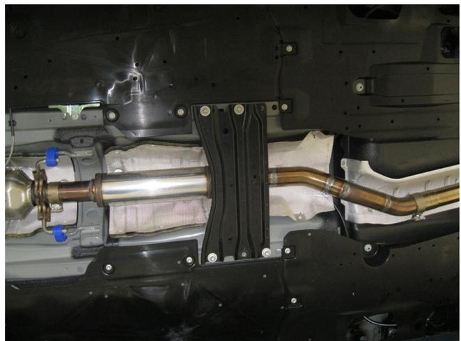
**Step 3.** Begin installation of your new MAGNAFLOW system by attaching the Resonator Assembly to the cut outlet behind the catalytic converter using the supplied 2.50" clamp. Keep all fasteners and clamps loose until final adjustment.
