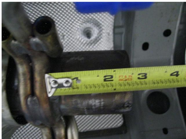
**Step 1.** Removal of this exhaust system requires cutting and de-burring the pipe 2.50" behind the hanger assembly welded to the pipe behind the catalytic converter. To accomplish this you must remove the cross brace and catalytic converter shield.
