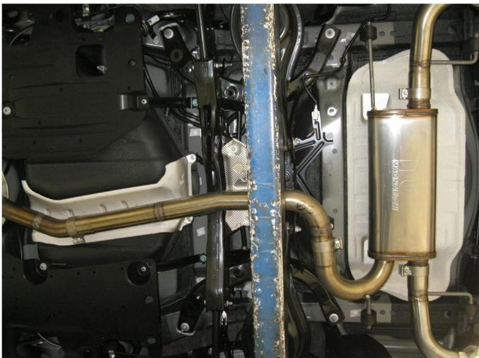
**Step 4.** Next use the supplied 2.50" clamps to attach the Mid-Pipe to the Resonator Assembly and the Muffler Assembly to the Mid Pipe. Insert hangers into rubber insulators.
