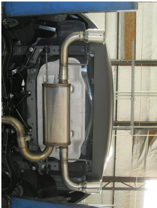
**Step 5.** Finish by attaching the Tail Pipe Assemblies to the Muffler with the supplied 2.50" clamps and fit hangers into rubber insulators.
