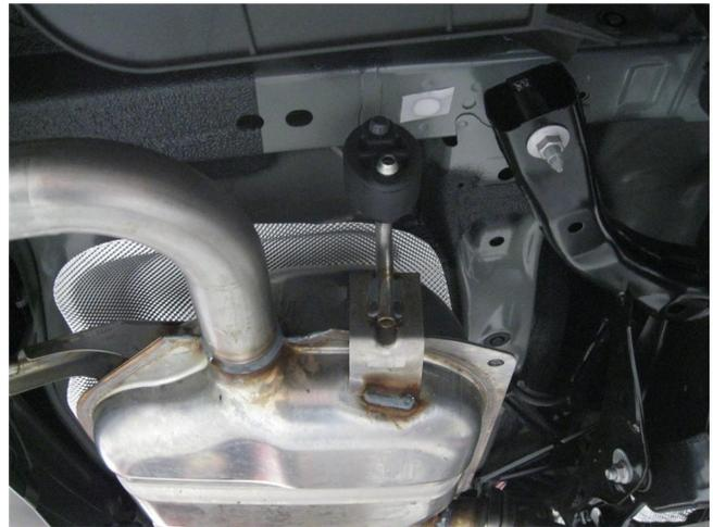
**Step 2.** Unfasten the flange at the rear muffler junction, disengage rubber insulators (Do not damage insulators as they will be used in the new installation).
