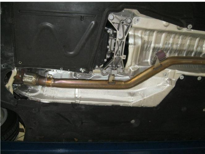
**Step 2.** Next, loosen the clamp attaching the inlet pipe to the flex pipe outlet. When removing the OEM system on this vehicle it is easier to unbolt the hanger assemblies with a #10 female TORX socket. The OEM exhaust system can now be removed in one piece. Retain all mounting hardware and rubber insulators as they will be needing to mount your new MAGNAFLOW system.
