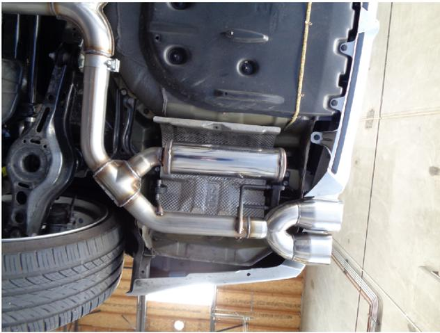
**Step 3.** Complete the installation by attaching the Muffler Assemblies to the Y-Pipe using the supplied 2.50" clamps. Engage the hangers into OE rubber insulators.
