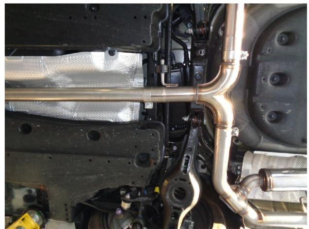
**Step 1.** To remove the OE exhaust system begin by unfastening the 2 bolt flange, working front to rear, (with the exhaust supported) disengage the hangers from the rubber insulators and remove the exhaust. Do not damage the rubber insulators and retain the front flange hardware as they will be used to install the new exhaust system.
