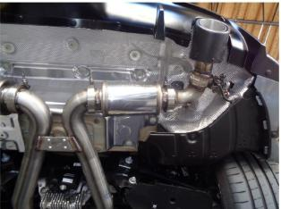
**Step 5.** Install the Muffler Assemblies (or Delete pipes) to the Extension Assemblies then attach the Tip Assemblies to the Mufflers using the supplied V-Clamps. Finish the installation by loosely attaching the MagnaFlow bracket between the Extension Pipes. Re-attach the valve wiring and OE cross brace.
