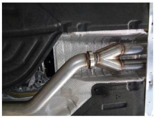
Step 3. MagnaFlow supplies this kit with multiple build options giving the ability to use different inlet pipe diameters and delete the mufflers depending on preference.
