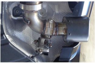
**Step 2.** Once the exhaust is off the vehicle remove the valve motor from the muffler assembly and transfer it over to the new exhaust valve assembly using the factory hardware.
