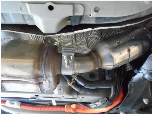
**Step 6.** Finish installation by tightening clamp and fasteners to torque specifications.
