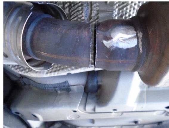
**Step 4.** Cut pipe at marked location. Loosen fasteners from inlet flange and remove converter. Clean and deburr cut pipe remaining on vehicle. (Retain fasteners to be used on installation of new MagnaFlow part)
