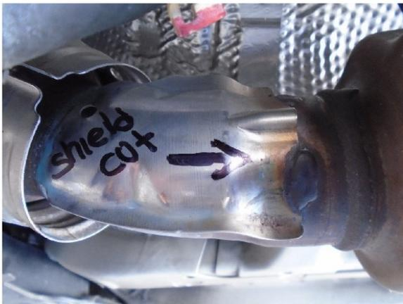
**Step 1.** Begin by Grinding (to remove) the weld attaching the heat shield to the converter pipe and remove the heatshield.
