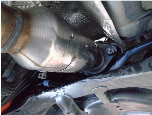
**Step 5.** Install the supplied clamp onto new MagnaFlow converter end and install over cut pipe on vehicle. Bolt converter flange into place using the OE fasteners.
