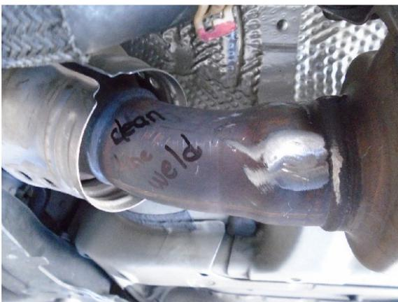
**Step 2.** Once heatshield is removed clean up weld burr.
