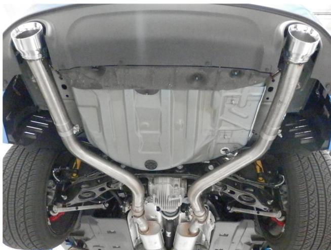
**Step 8.** Loosely attach each Tail Pipe Assembly to the Mid Pipes using the supplied clamps. Engage the welded hangers for each to the rubber insulators.
