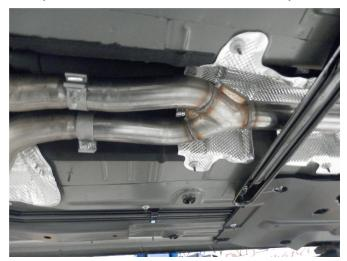
**Step 2.** Begin installation of the new system by attaching the Inlet Pipe Assembly to the outlets of the OEM system using the supplied 2.25" clamps. Leave all clamps loose for final adjustment.
