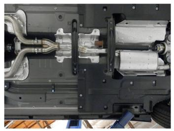
**Step 1.** To allow for removal of the OEM exhaust you will need to remove the underbody braces. Begin the removal of the OEM system by unfastening the inlet pipe inlets at the factory clamp locations. Un-clip the ground strap from the passenger side hanger and working rearward (with the exhaust supported) extract the hangers from the rubber insulators and remove the OEM exhaust. Do not discard or damage the rubber insulators as they will be used to install the new exhaust system.
