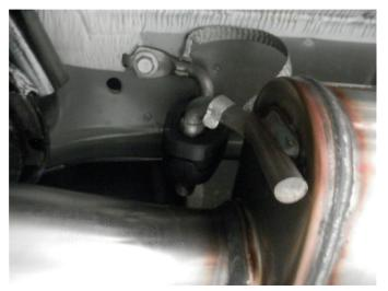
**Step 5.** Re-attach the ground strap to the hanger. Finish the installation mounting underbody braces.
