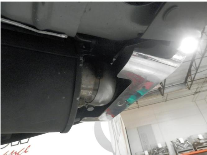
**Step 3.** Next, loosen the band clamps attaching the rear mufflers to the OEM tips. You may now remove the rear exhaust system. Disengage all welded hangers from the rubber insulators. Once the two mufflers are removed from the vehicle detach the OEM tip clamps by gently breaking the welds securing them. Do not discard or damage the clamps or rubber insulators as they will be used to install the new exhaust system.
