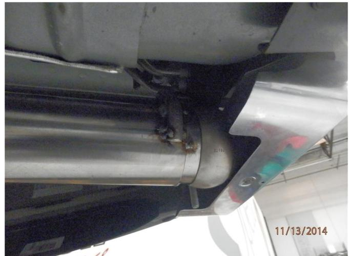
**Step 5.** To retain the OEM tips on your vehicle select the two OEM Tip Assemblies. The drivers side will be slightly longer. Loosely attach each pipe inlet to the Over Axle Pipes outlets using the OEM clamps. Engage the welded hangers for each to the rubber insulators.
