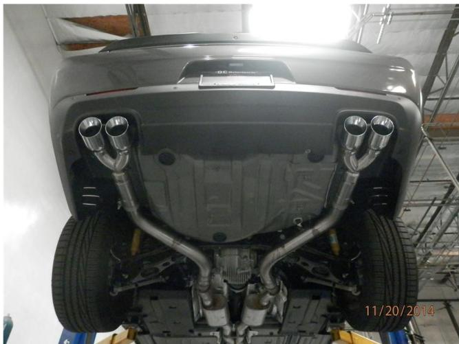
**Step 7.** Once the tips are removed install the Quad Tip Tailpipe Assemblies using the supplied 3.00" clamps. Locate both welded hangers to the rubber insulators.
