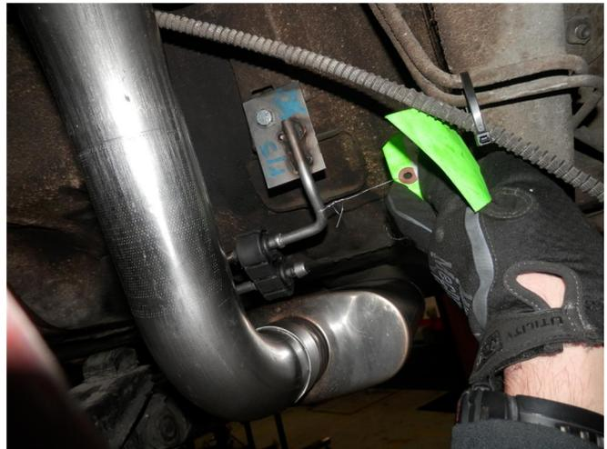
**Step 3.** Use supplied Hanger Brackets to mount both Muffler Assemblies. Secure using the supplied hardware.
