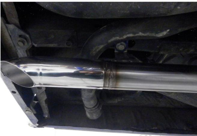
**Step 7.** Lastly, install both Polished Tips to the Tail Pipes. Once in the desired position weld each tip as shown.
