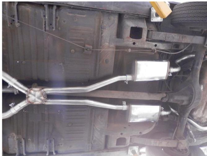
**Step 2.** Loosely attach the X-Pipe Assembly to the Inlet Pipes and then the Muffler Assemblies to the X-Pipe Assembly using the supplied clamps.
