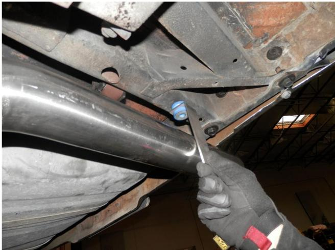
**Step 6.** Secure the Tail Pipes with the supplied Tip Hanger Brackets and Snap Grommets. Try to position each bracket to locate an existing hole in the vehicles sub frame to avoid drilling. Once the desired position has been found mark its location. Trim the bracket as necessary and bolt the bracket with the Snap Grommet to the sub frame using the supplied hardware. Weld the bracket to the Tail Pipe once you have the pipe in position.
