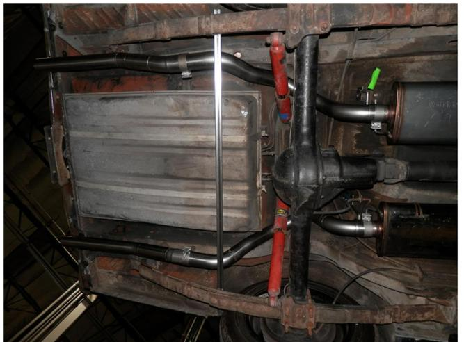
**Step 5.** Next, loosely attach the desired Tail Pipe Options using the supplied clamps.
