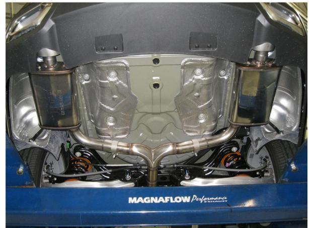
**Step 4.** Finish by installing the Muffler Assemblies to the Y-Pipe Assembly using the supplied 2.50" clamps, and fitting the welded hangers into the rubber insulators.
