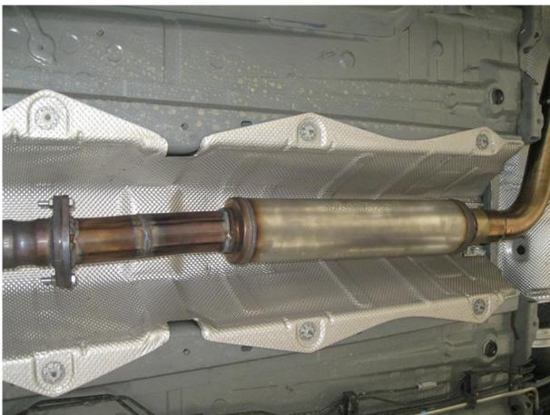
**Step 2.** To begin, fasten the Resonator Assembly inlet to the catalytic converter using the provided fasteners and gasket (Leave all clamps and fasteners loose for final adjustment of the complete system.)
