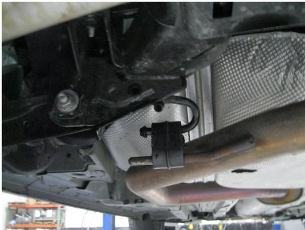
**Step 1.** To remove the OEM exhaust system, you will first need to unbolt the resonator from the catalytic converter and disengage all welded hangers from the rubber insulators. Do not damage or discard the rubber insulators, as they will be reused to mount the new system. You can now remove the exhaust from the vehicle.
