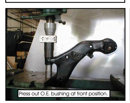
Press out O.E. outer metal shell from aluminum bracket, then press pivot pin on control arm out of bushing. A pressed fit sleeve will then need to be removed. Grease all metal parts that will touch bushing # 3447. Part numburs faces the rear.
