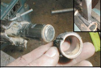
The sleeve will need to come off the rear pin. It's a tight press fit. With a hammer and chisel, make a groove along its length, this will relieve the press fit. The sleeve will then slide off by hand.
